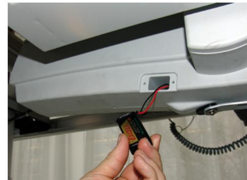
Then pull the contact strip off the battery.
