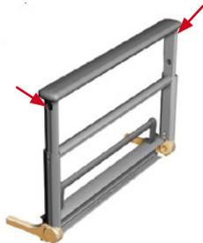
2. Press the "Drücken / Push" trigger at the lower edge of the side rail element and tilt it sideways into the horizontal plane, so that it lies parallel to the floor.
