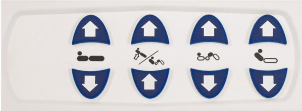
Lying surface down    Auto-Contour<sup>2</sup> (optional)    Upper leg section down    Back section down
