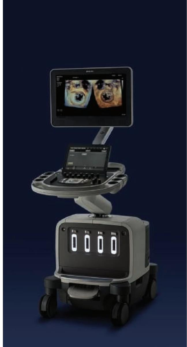
Easy viewing and efficient use even in darker scanning environments with a large 54.6 cm (21.5 in) wide screen and ambient lighting that provides subtle visual cues for the keyboard, OEMS, and transducer ports. Four transducer ports decrease the amount of plug/unplugging required during a day of scanning.
