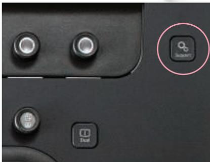
Service Request button for immediate access to Philips support.
