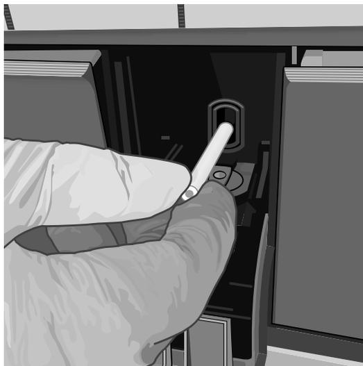
**Figure 72. Inserting the Cleaning Brush into the I-CORE Module Slit**
