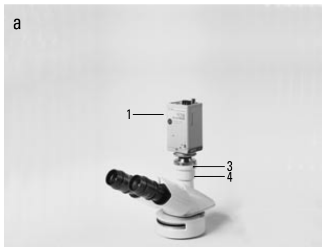
Fig. 34 C-mount adapter on trinocular tube
