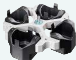
Swing-out rotor, 4-place illustrated with carriers 4486-R n = 4,500 \text{ min}^{-1} , max. RCF = 4,392
