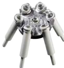
Swing-out rotor, 6-place, for chrome bath tubes n = 2.000 \text{ min}^{-1} , max. RCF = 917
