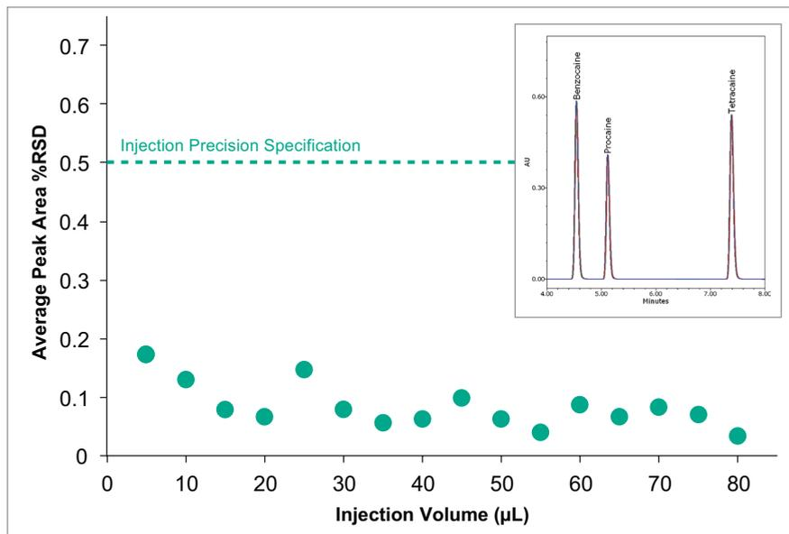
Average peak area %RSD for six replicate injections is plotted as a function of injection volume. Across the entire volume range, the injection precision is below 0.2% and well below instrument specification. Inset shows and overlay of six replicate injections at 50 µL.
