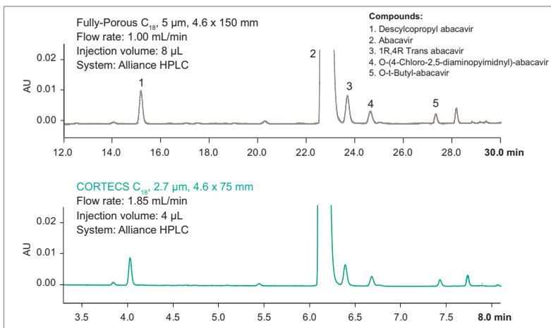
*The method for Abacavir is transferred from a fully porous 5 µm C<sub>18</sub> to a CORTECS C<sub>18</sub> 2.7 µm with a 4x reduction in run time and equivalent resolution, both on an Alliance HPLC System.*
