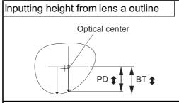
This is the form to input the height of the optical center by measuring the distance from the eye point to the bottom of the lens outline.
