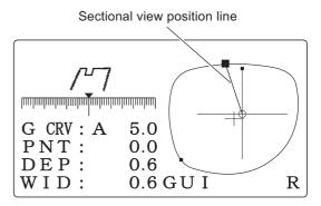
: The sectional view position line jumps to the point that the lens edge is thinnest ( $\blacksquare$ ) and thickest (**a**) alternately.
