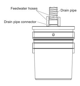
10. Attach a new stocking filter to the drain pipe connector.
