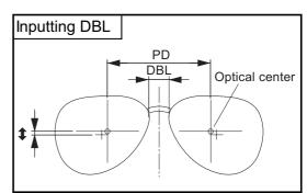
This is the form to input DBL (distance between the nasal ends of the right and left rims) instead of FPD.
