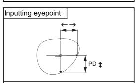
This is the form to input the eyepoint as the optical center by the distance measured from the nasal and bottom sides of the lens outline.
