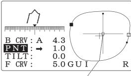
Set the tilt base position near the point straight down from the frame center.
