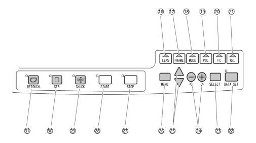
Selects a lens material; PLA (plastic), HPL (high index plastic), PC (polycarbonate), GLS (glass), ACR (acrylic resin) or TRX (trivex). (For Type PLB, GLS cannot be selected.)
