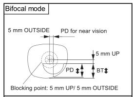
This is for bifocal lenses. Block at the position of 5 mm above and 5 mm outside from the top line center of the segment with a lens cup.
