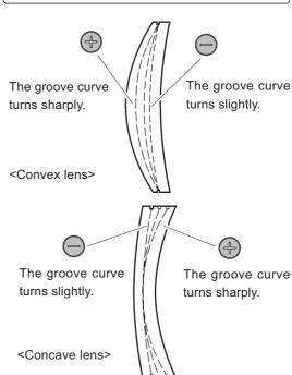
The curve value with the "A" mark on the head shows that it is a computer-calculated value. This value produces the same groove curve that is processed in the auto grooving mode.
