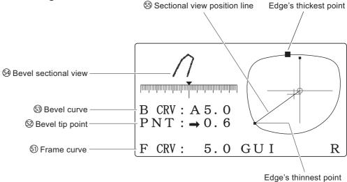
This screen is shown while a bevel is simulated (when the tilting function is ON).
