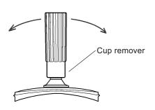
Since lenses such as polycarbonate lenses are thin, prying the cup may crack the coated surface of the lens. In such cases, remove the lens cup while turning the remover.
