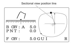
5. Simulate the bevel section at each point of the traced outline on the screen.
