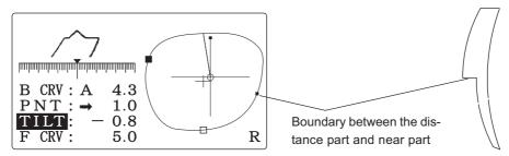
See the following in adjusting the bevel position at each point. To reset all the settings, reset "TILT" and "PNT" to 0.0, and put "A (automatically-calculated curve value)" at the head of the curve value. This will allow an operator to reset the bevel position and tilting amount from the beginning.
