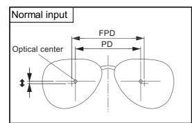
This is the form to input FPD, PD and the height of the optical center from the center of the rim ( ‡ ).
