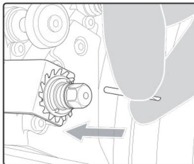
7 Put the adjustable wrench onto the chuck, then tighten (two notches towards the bottom of the trough).
