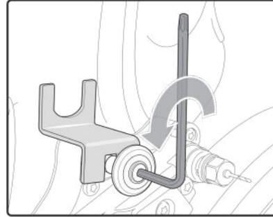
6 Remove the chamfering wheel and the spacer.
