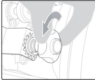
5 Remove the adjustable wrench then the mill bit.
