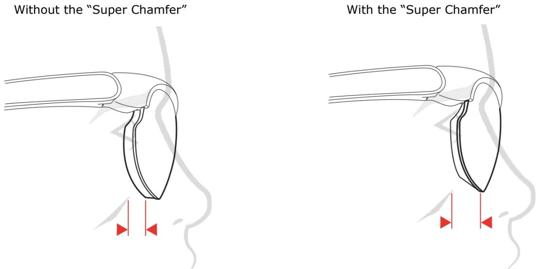
The "Super Chamfer" allows you to break the ridge of the lens on the rear surface at a defined distance and configure it in relation to:
