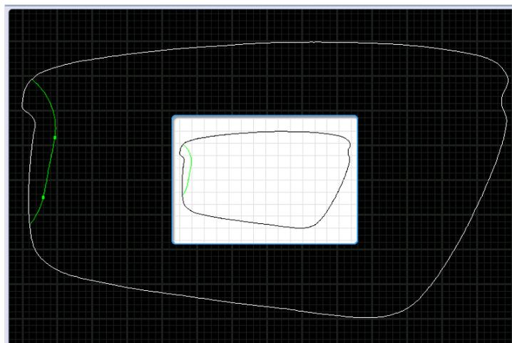
4 Press and hold with the stylus to set the other points of the step bevel trajectory, one after the other.
