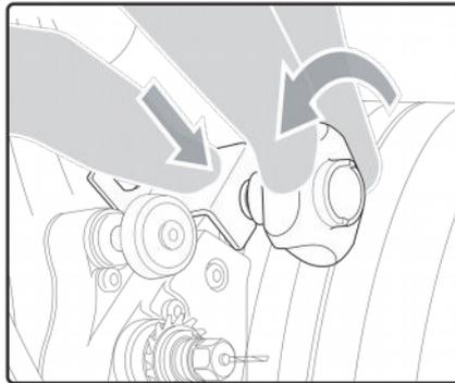
**4** Remove the adjustable wrench then the drill bit.
