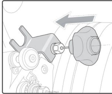
**3** Loosen the chuck with the adjustable wrench (two notches towards yourself).
