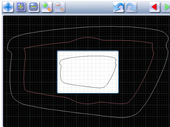
2 Press and hold the stylus to set the first point of the step bevel trajectory.
