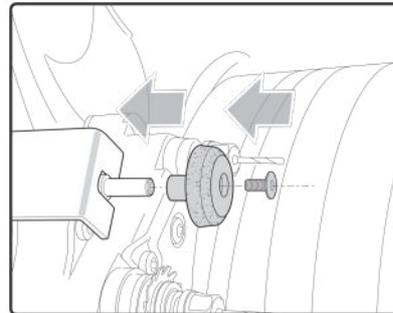
8 Tighten (towards yourself) the "step ++" wheel using the torque wrench.
