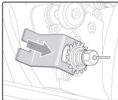
3 Put the adjustable wrench on the chuck
