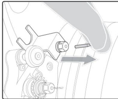
**5** Insert the engraving tip all the way, then tighten the chuck firmly by hand.
