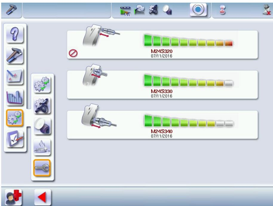
The bargraph flashes and the icon
