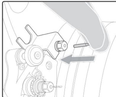
**8** Tighten the chuck with the adjustable wrench (two notches towards the back of the trough).
