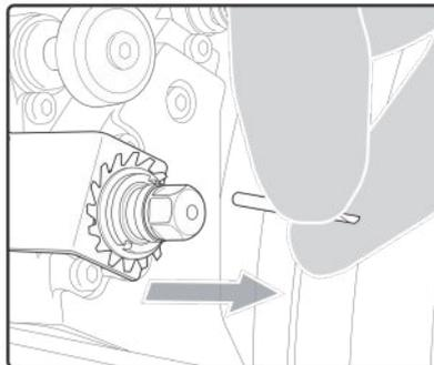
6 Inset the new mill bit all the way at the back.
