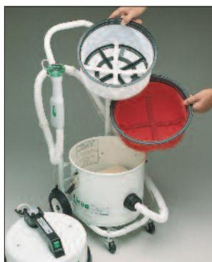
The four stage filtration system consisting of an easy to change disposable collection bag, two cloth filters and a micro filter. The micro filter retains 99.997% of all dust particles greater than 0.5 microns.
