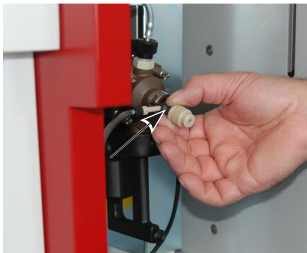
Fig. 60 Withdrawing the nebulizer from the mixing chamber
