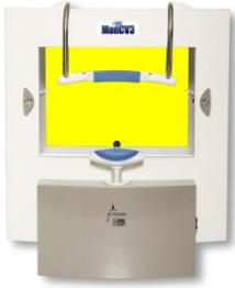
The apparatus can generate blue color tests with Goldmann size V which are projected over a high luminance yellow background ( $100 \text{ cd/m}^2$ ), for the detection of early glaucoma deficits.
