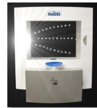
For the glare test, the instrument is equipped with sources of very high luminance ( $> 20\,000 \text{ cd/m}^2$ ) positioned on the side of the screen.
