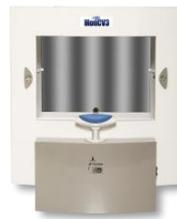
The contrast sensitivity tests are performed with sinusoidal gratings with controlled spatial frequencies, luminance and contrast.
