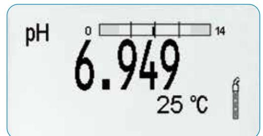
The CMC function (Continuous Measurement Control) of a pH 3310 informs you whether you are measuring inside the calibrated range. An alert is given as soon as you are outside the limits.
