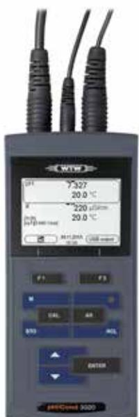
The pH/Cond 3320 has a robust waterproof housing (IP 67) and is equipped with a large memory and a data logging function with an adjustable interval between 1 s and 60 minutes. All records have a time and date stamp as well as an assignable ID number. The waterproof USB interface makes data transfer fast and easy.
