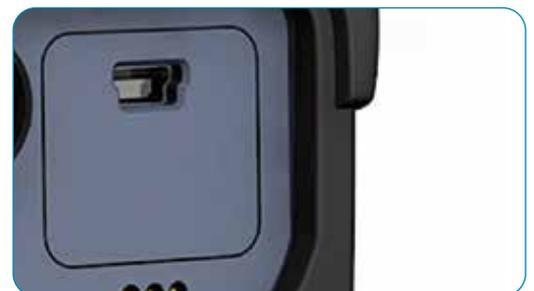
100% waterproof USB interface for fast communication with a PC or laptop.
