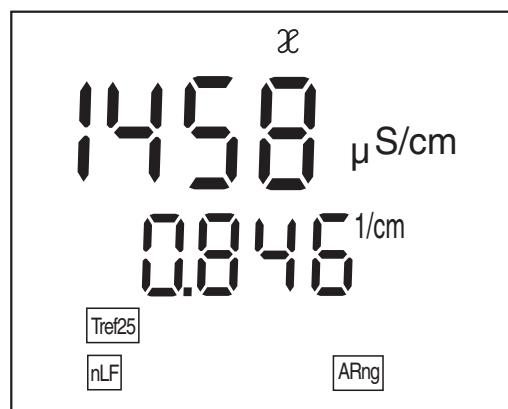
5 Confirm the selection with <ENTER>. The new cell constant is used from now on. The meter switches to the measured value display.
