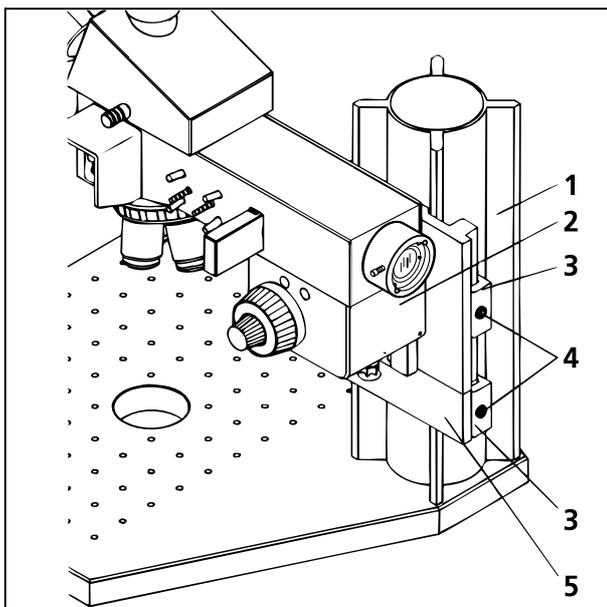
Fig. 2-4 Axiotech<sup>vario</sup> - Attaching the microscope body to column X95
