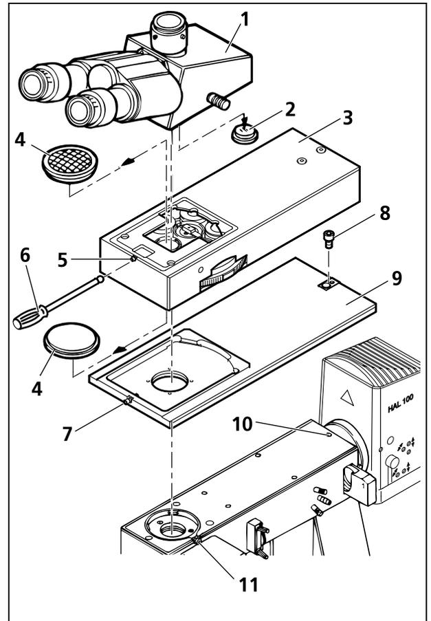
Fig. 2-8 Attachment of Optovar intermediate tube
