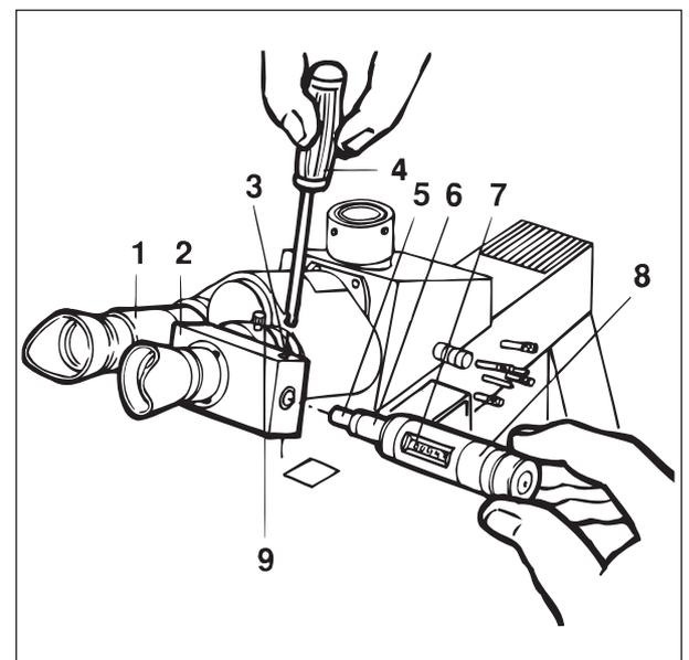
Fig. 3-35 Attachment of digital eyepiece measuring device
