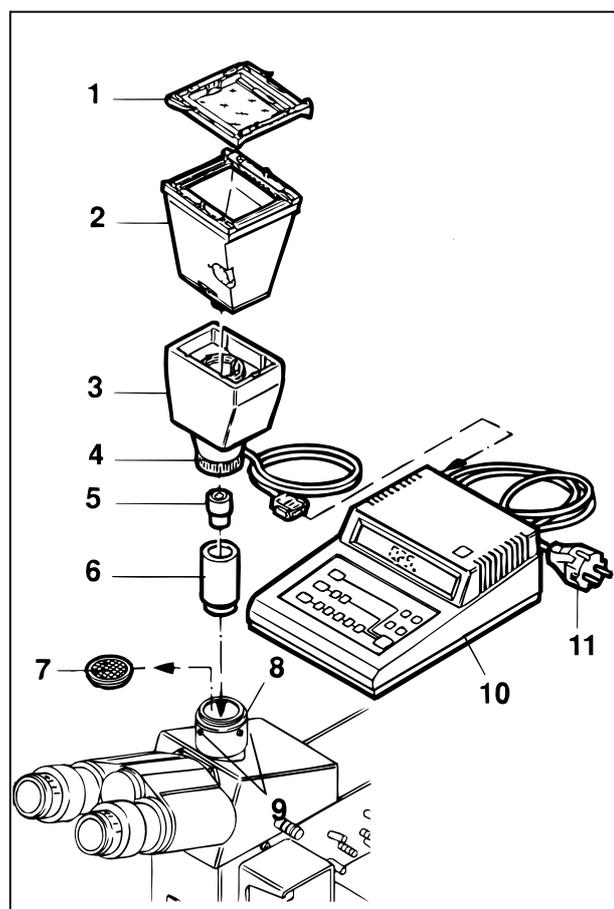
**Fig. 3-31 Attachment of MC 80 DX microscope camera (large format)**
