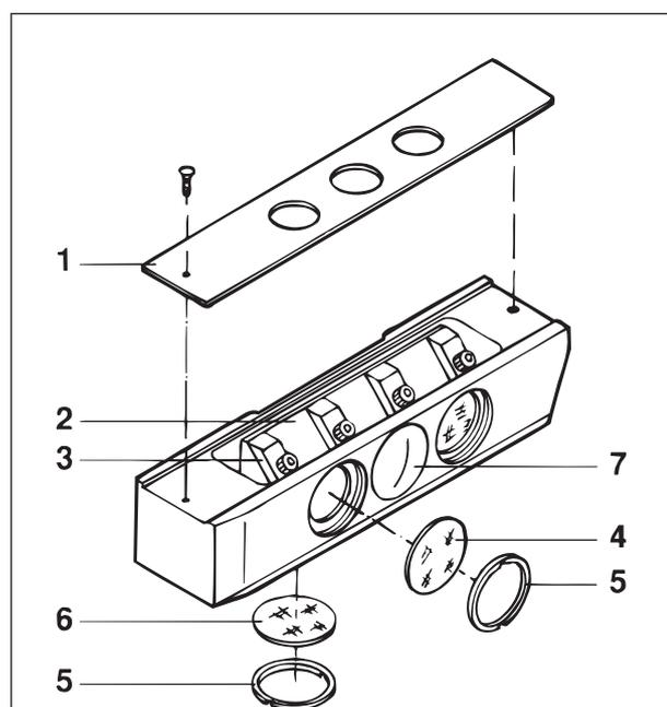
**Fig. 3-18 3 FL reflector slider**
