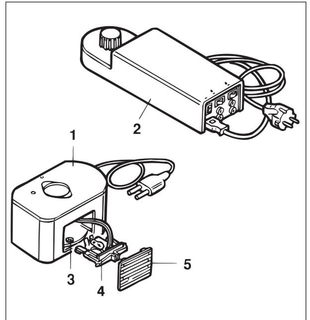
**Fig. 2-34 Change of 6 V 30 W halogen lamp
