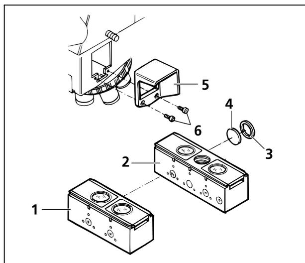
Fig. 2-21 Change of filters in reflector slider
