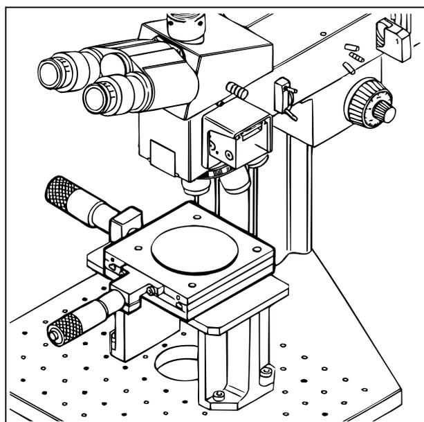
Fig. 2-18 Specimen stage MT 50 x 50
