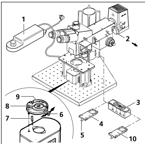
**Fig. 3-24 Setting of transmitted-light polarization contrast with reflector slider HD DIC (Axiotech<sup>vario</sup> 100)**
