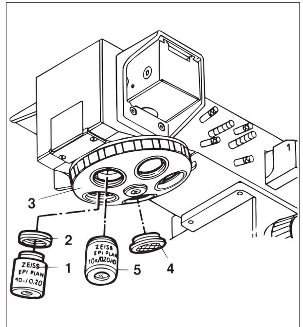
Fig. 2-5 Screw in objectives
