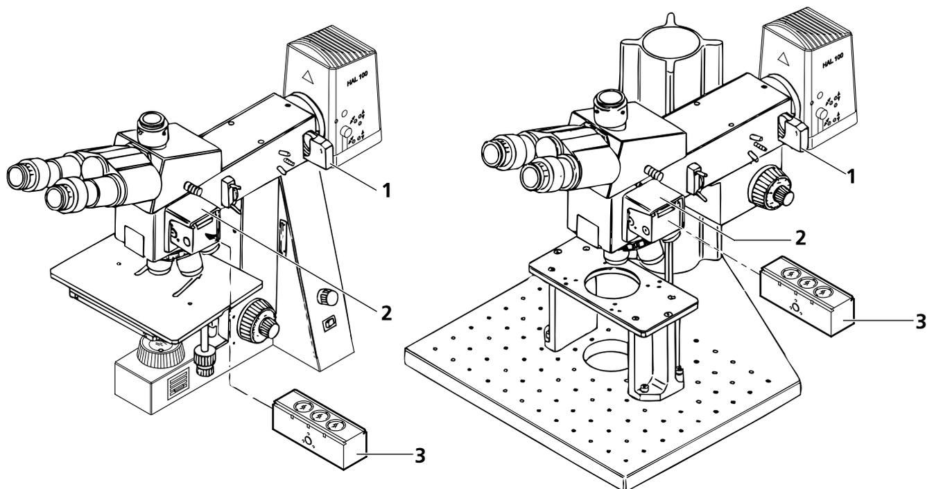
**Fig. 3-17** Setting of epi-fluorescence using the 3 FL reflector slider
