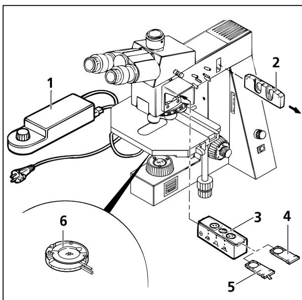
**Fig. 3-22** Setting of transmitted-light polarization contrast with reflector slider HD DIC (Axiotech 30/100)
