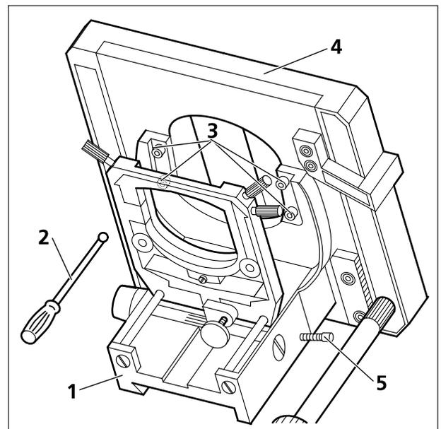
Fig. 2-16 Attachment/change of microscope stage (configuration with stage carrier D)
