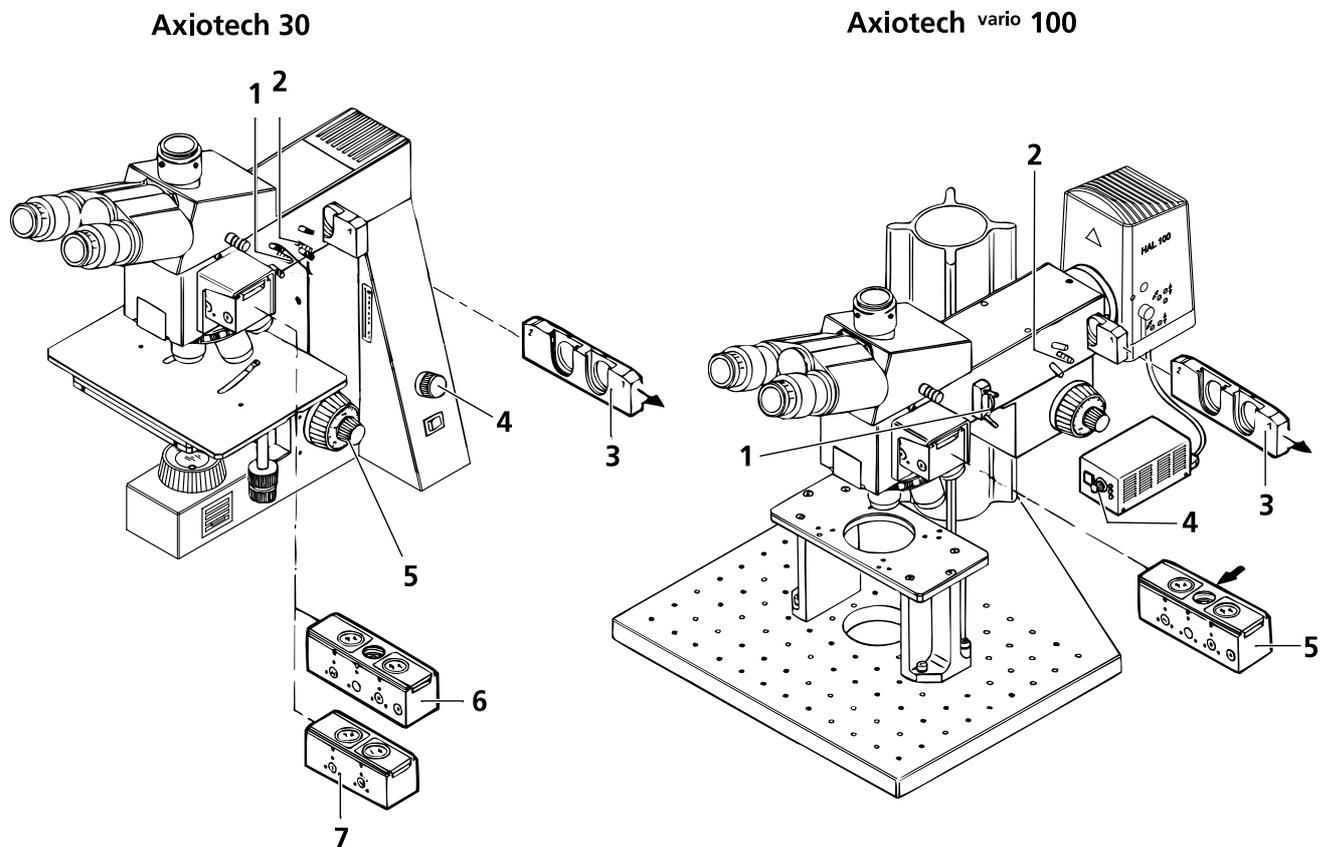
**Fig. 3-10 Setting of reflected-light darkfield**
