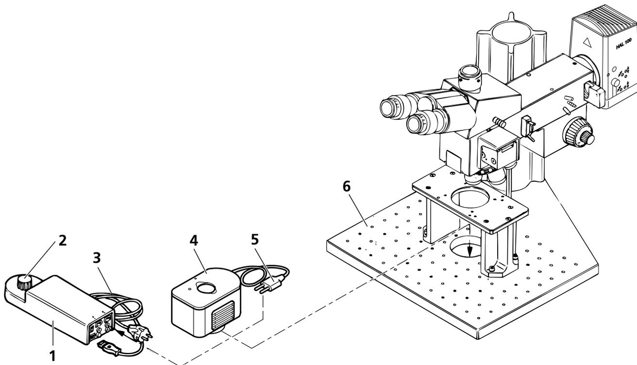
Fig. 2-35 Connection of power supply for 6 V 30 W halogen illuminator (Axiotech<sup>vario</sup> 100)
