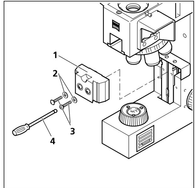
Fig. 2-15 Attachment of adapter for stage carrier D
