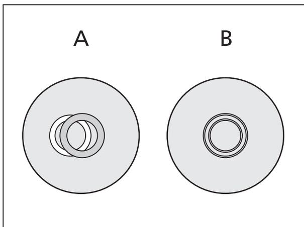
**Fig. 3-28** Centering of phase stop (bright in condenser) with phase ring (dark in objective)
