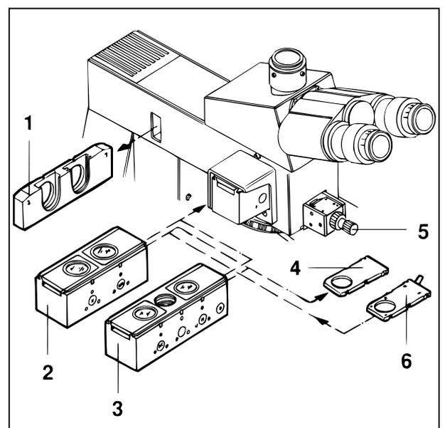
Fig. 3-14 Setting of reflected-light polarization contrast
