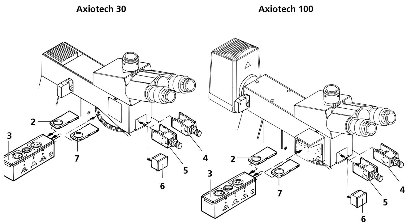
**Fig. 3-12 Setting of reflected-light interference contrast**
