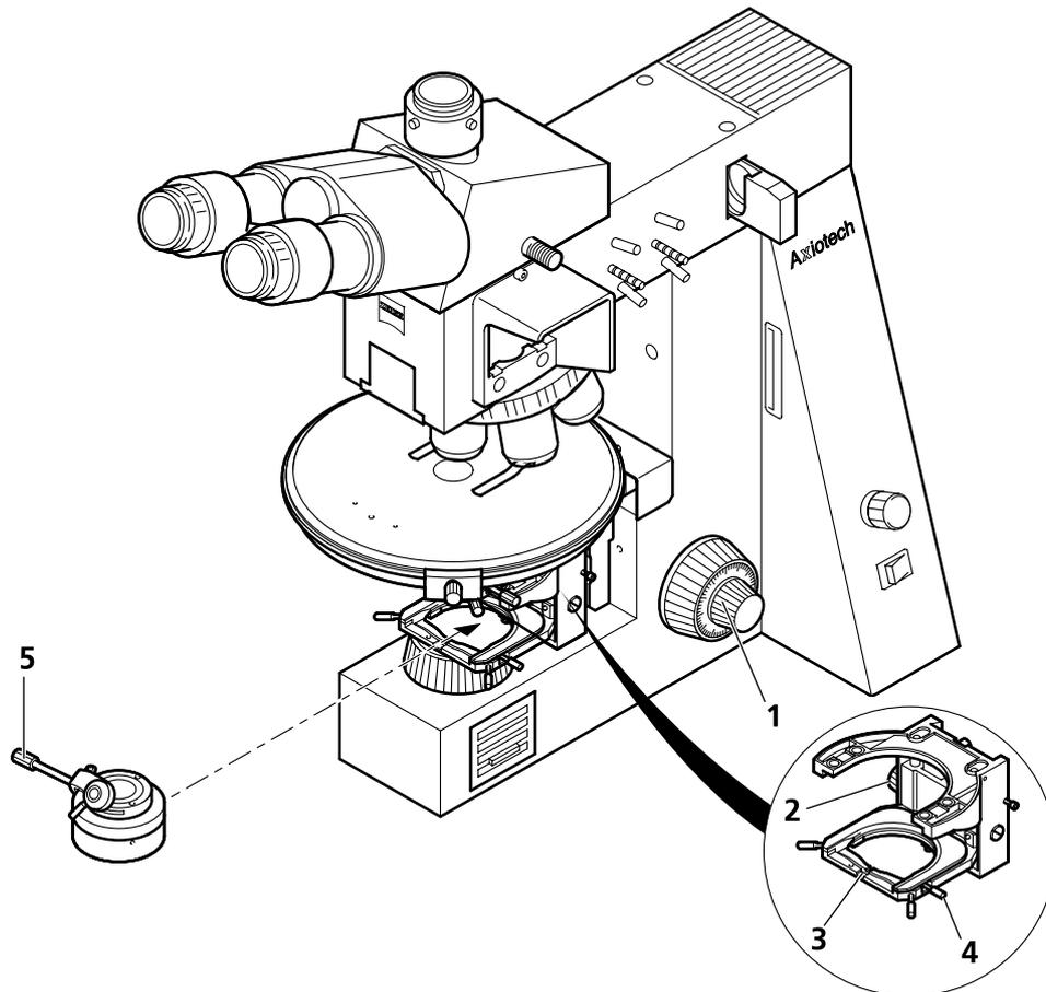
**Fig. 2-13 Attachment of condenser**
