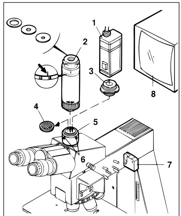
**Fig. 3-32 Attachment of video camera**
