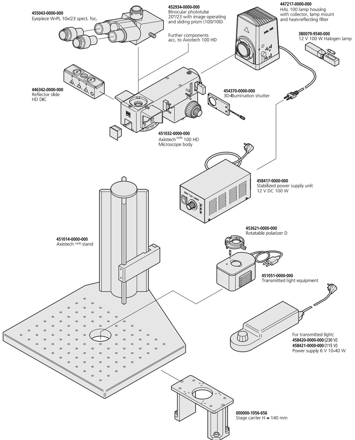
Fig. 1-5 Microscope components and modules (sheet 5)
