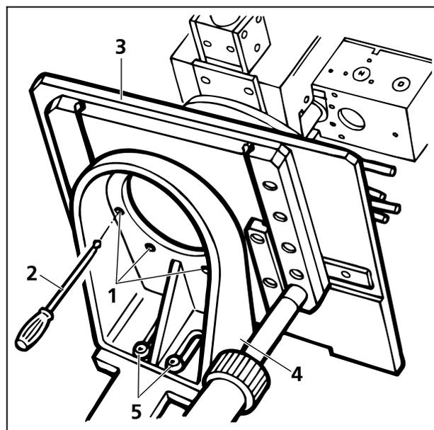
**Fig. 2-14 Attachment/change of microscope stage (configuration with stage carrier A)**
