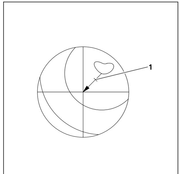
**Fig. 2-19** Centering of microscope stage with maximum deflection between object detail and eyepiece reticle
