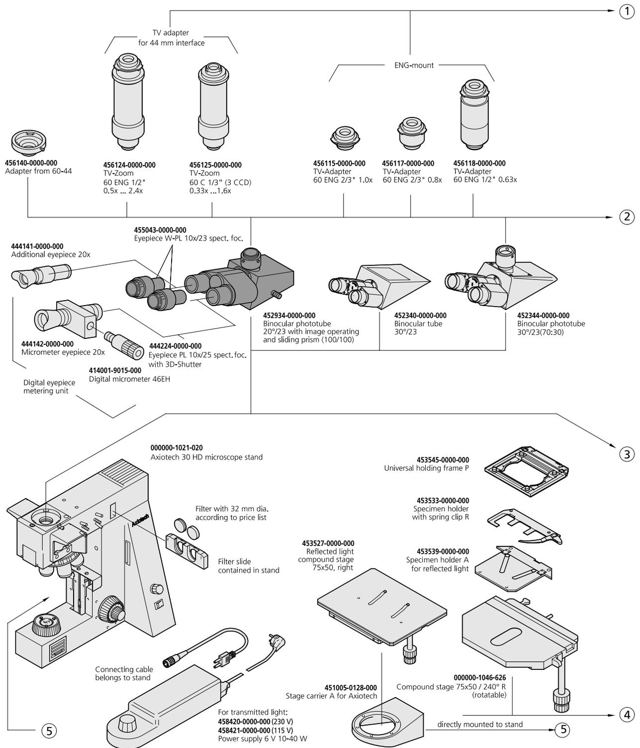
Fig. 1-1 Microscope components and modules (sheet 1)
