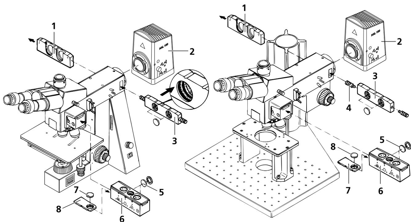
Fig. 3-16 Setting of epi-fluorescence using the FL filter slider
