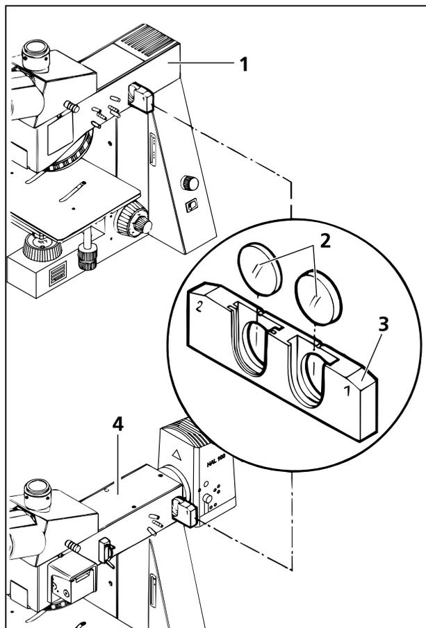
Fig. 2-20 Equip filter slider and push it in beam path
