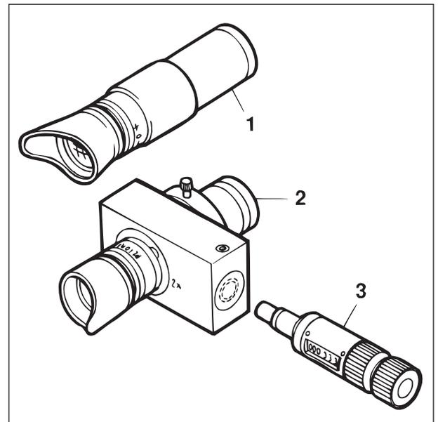
Fig. 3-34 Digital eyepiece measuring device
