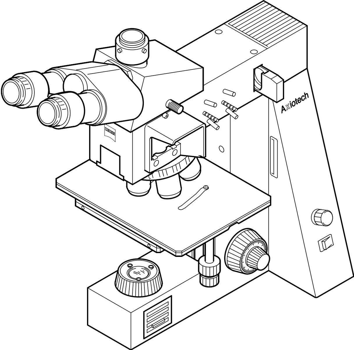
Overall view of the Axiotech 100 reflected-light microscope
