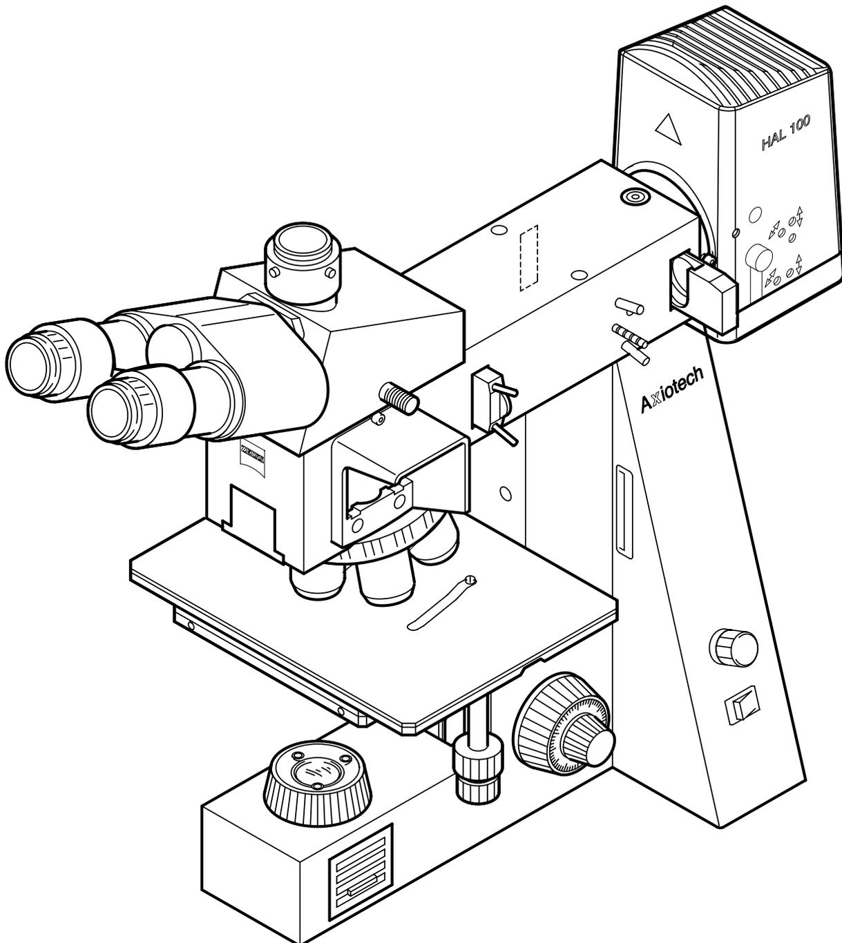
Overall view of the Axiotech<sup>vario</sup> 100 reflected-light microscope
