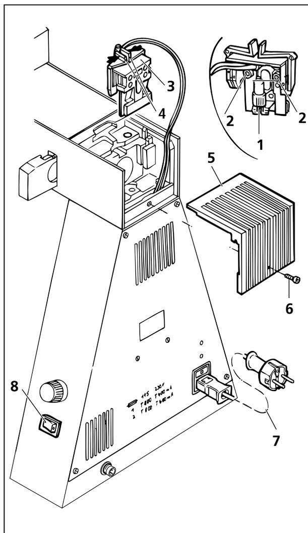
Fig. 2-28 Change of 6 V 30 W halogen lamp
