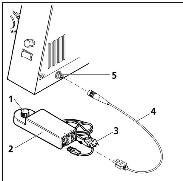
**Fig. 2-33 Connecting the 6 V 30 W halogen illuminator to the line**
