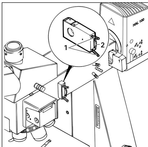
Fig. 2-23 Setting of reflected-light luminous-field diaphragm on Axiotech 100 and Axiotech<sup>vario</sup> 100
