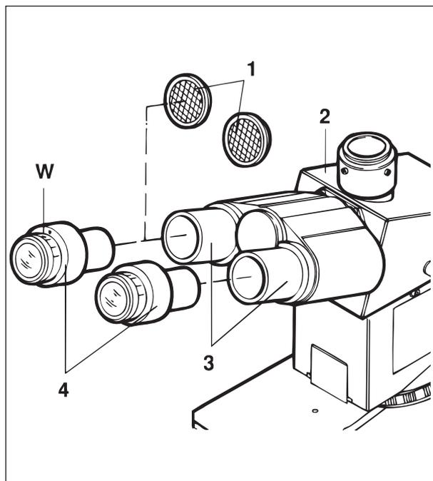
Fig. 2-9 Insertion of eyepieces
