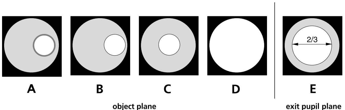
**Fig. 3-8** Setting of diaphragm images according to KÖHLER
