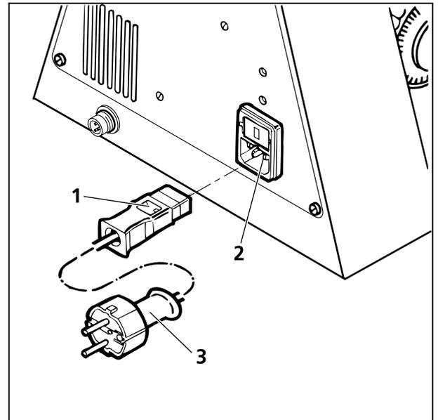
Fig. 2-24 Connecting the Axiotech 30 to the line
