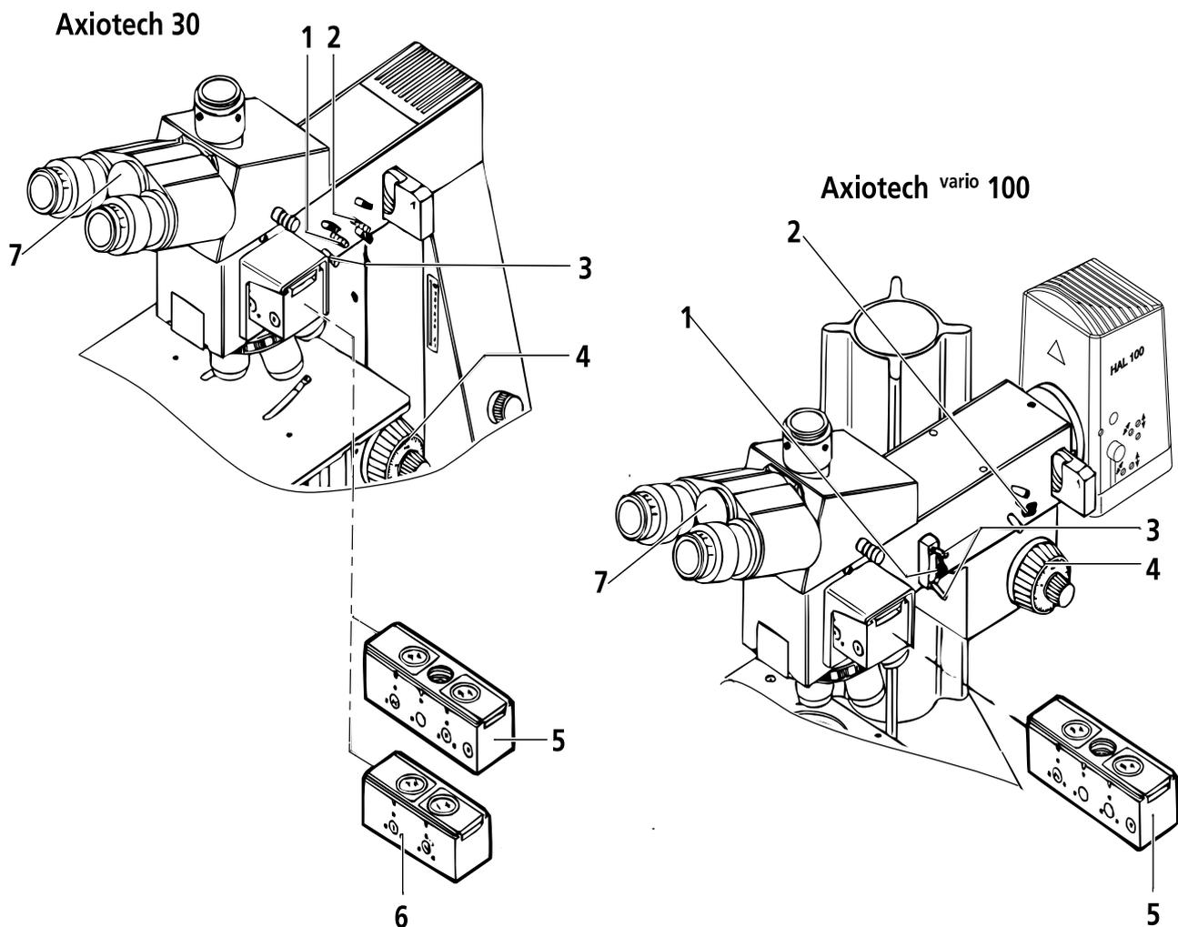
**Fig. 3-7** Setting of reflected-light brightfield
