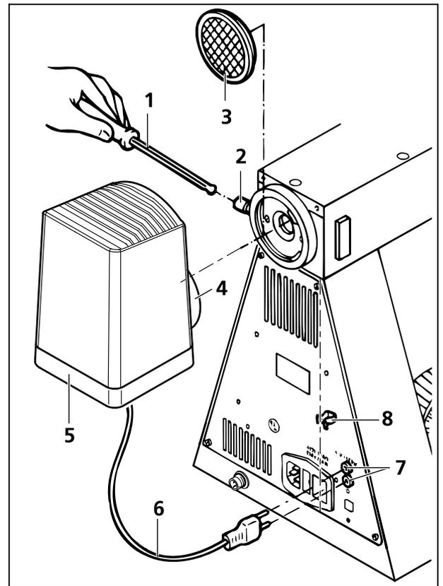
Fig. 2-29 Attachment of 12 V 100 W halogen illuminator
