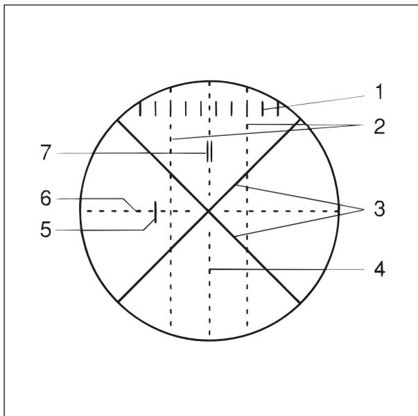
**Fig. 3-36** Crossline figure in the eyepiece intermediate image of the digital eyepiece measuring device
