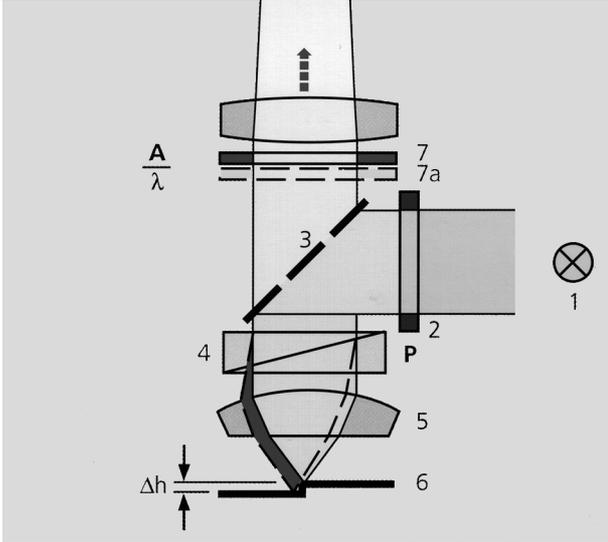
**Fig. 3-11 Reflected-light interference contrast**
