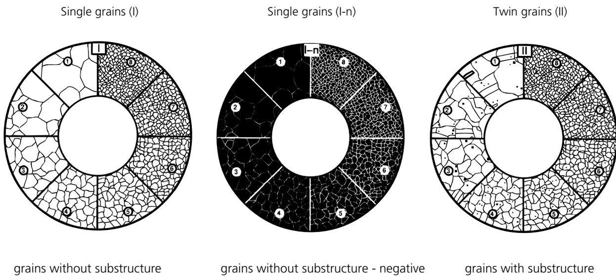
**Fig. 3-38** Structure comparison reticles
