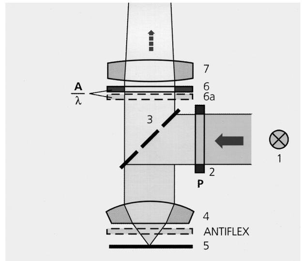
Fig. 3-13 Reflected-light polarization contrast
