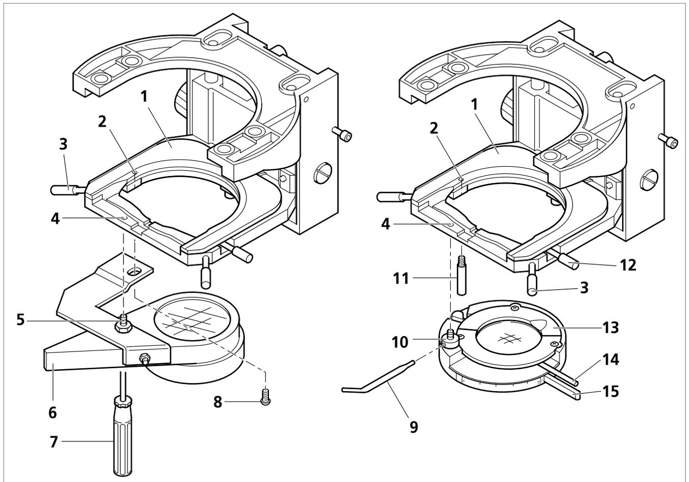
**Fig. 3-23 Attach polarizer to stage carrier D**
