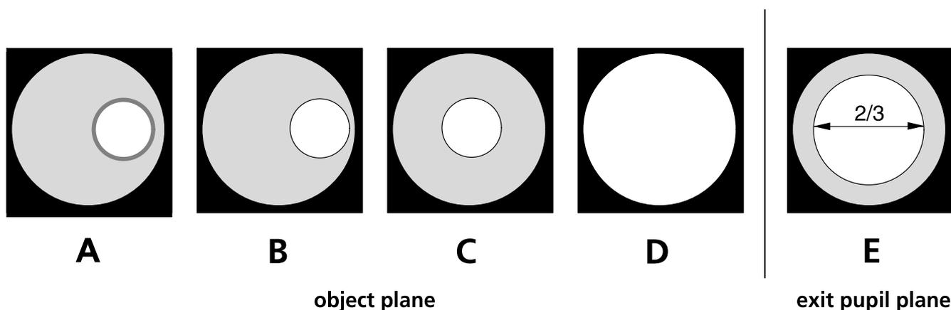
Fig. 3-20 Setting of diaphragm images according to KÖHLER
