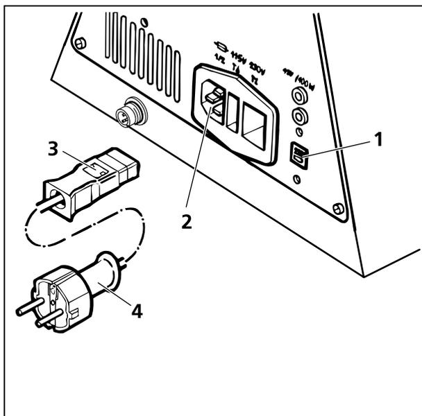
Fig. 2-26 Connecting the Axiotech 100 to the line
