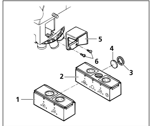
**Fig. 3-19** Change of filters in the reflector slider
