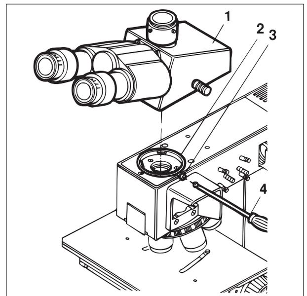
Fig. 2-6 Attachment of binocular tube
