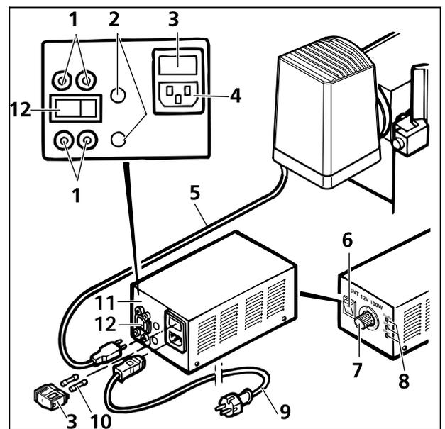
Fig. 2-27 Connecting the Axiotech<sup>vario</sup> 100 to the line via separate power unit
