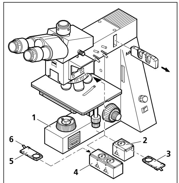
**Fig. 3-25** Setting of transmitted-light polarization contrast using reflector slider without DIC position (Axiotech 30/100)
