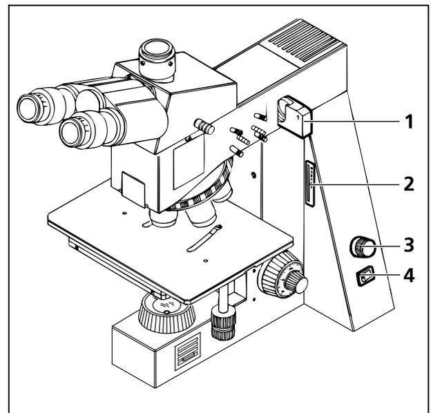
Fig. 2-25 Switching on the Axiotech 30
