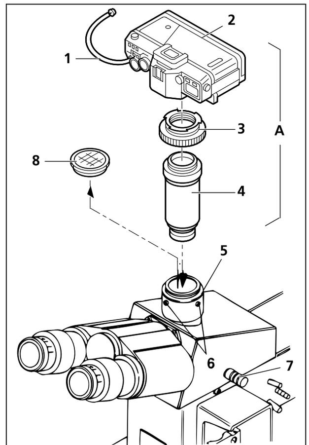
Fig. 3-29 Attachment of SLR camera, e.g. CONTAX Aria
