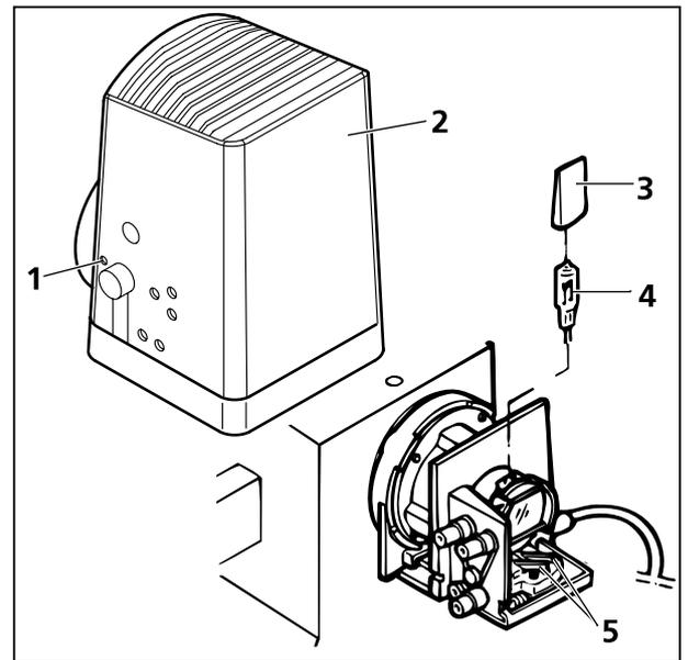
**Fig. 2-31** Change of 12 V 100 W halogen lamp
