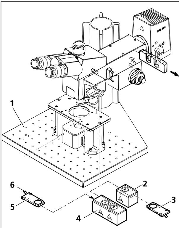
**Fig. 3-26** Setting of transmitted-light polarization contrast using reflector slider without DIC position (Axiotech<sup>vario</sup> 100)
