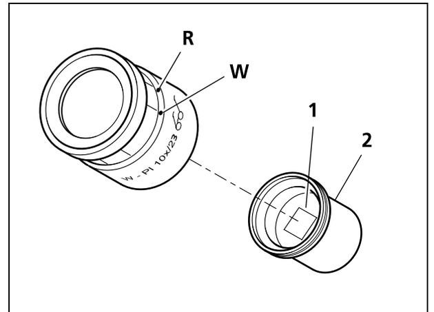
Fig. 2-11 Insertion of the eyepiece reticle
