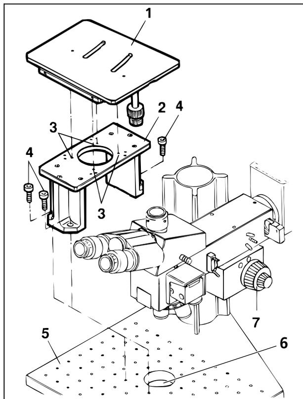
Fig. 2-17 Attachment/change of microscope stage (stage carrier H = 140 mm)
