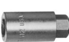
870432 Socket, for tightening titanium caps (cap 341968), 7/16-in. (11 mm) hex nut
