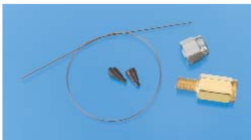
Figure 1 The EZ No-Vent™ connector incorporates a laser machined orifice for optimal flow through the fitting. Coupled with the 100µm ID transfer line, it minimizes the amount of oxygen entering the MS, which eliminates the need for purge gases.
