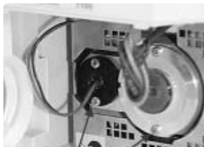
Step 1: Remove the lamp by unscrewing both screws and unplugging it.
