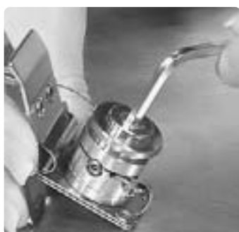
Step 3: Remove the cell screw and remove the gasket
