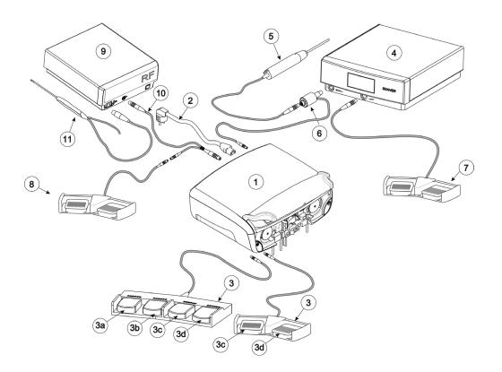
1 Double Pump RF 4 ) Shaver console 5 Shaver Hand piece 2 Mains Cable ) Foot Control: Shaver Interface Box A 4 pedal or 2 pedal Foot Control may be Shaver Foot Control used: a) Shaver Reverse 8 RF Generators Foot Control b) Shaver Forward c) Cannula ) RF Generαtor d) Rinse (10) RF Cable A2 (11) RF Probe
