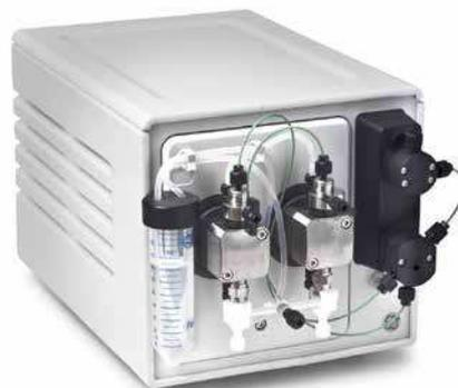
**Fig 4.** ÄKTA pure sample pump.
