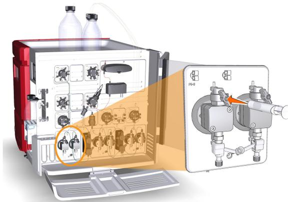
7 Open the purge valve by turning it counter-clockwise about three-quarters of a turn. Draw 5 to 10 ml of liquid slowly into the syringe with a rate of about 1 ml/s.
