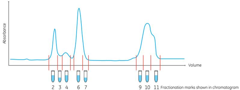
When peak fractionation is used, Fraction collector F9-R collects the delay volumes in the fractions preceding each peak. In the chromatogram above, delay volumes are collected in tubes corresponding to fraction 1, 5 and 8. The numerical fraction marks for the delay volume fractions are not indicated on the chromatogram.
