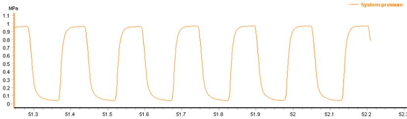
**Incident:** Inlet check valve is loose.
