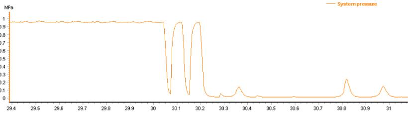
**Incident:** Blocked outlet check valve
