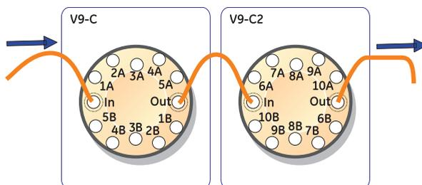
**Note:** The standard Column valve (**V9-C** or **V9H-C**) must be connected before the second Column valve (**V9-C2** or **V9H-C2**). Otherwise, the pressure monitors will not function correctly.
