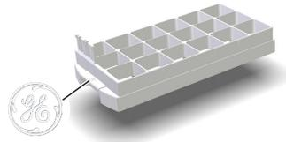
**Note:** The tray and racks are inserted into the fraction collector with the GE monogram facing outwards.
