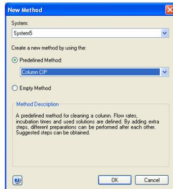
*Result:* One **Method Settings** phase and one **Column CIP** phase will be displayed in the **Method Outline** pane.
