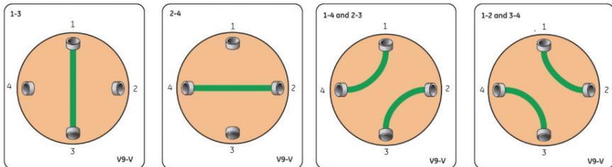
The Versatile valve has four available sets of flow paths; two where a single flow channel is used and two where the flow can be directed through two different channels simultaneously.
