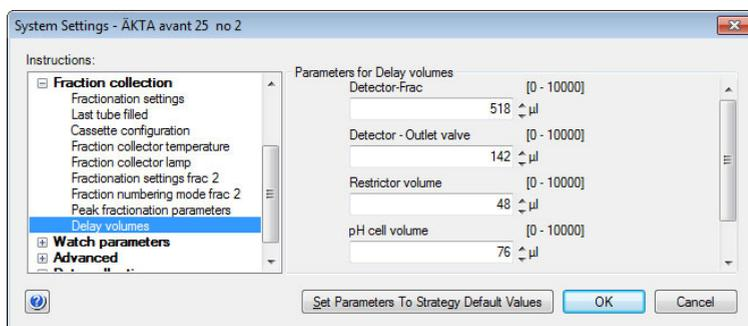
**Note:** The system will use the delay volume appropriate to the configuration used and ignore other settings (e.g. the value for **Detector-Outlet valve** will be ignored if you are using a fraction collector). It is however recommended to set all delay volumes so that the volumes remain correct if you change fractionation method.
