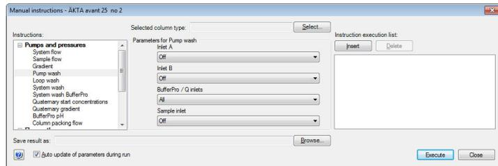
**Result:** A simultaneous pump wash of all the Q inlets is started. This will remove air from Quaternary Valve.
