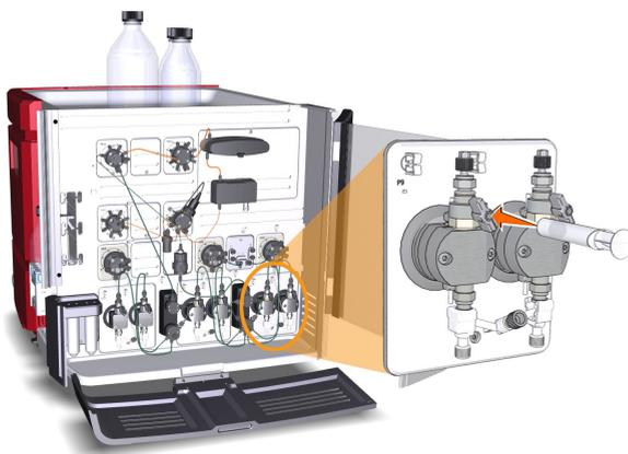
5      Open the purge valve by turning it counter-clockwise about three quarters of a turn. Draw liquid slowly into the syringe until the liquid reaches the pump.
