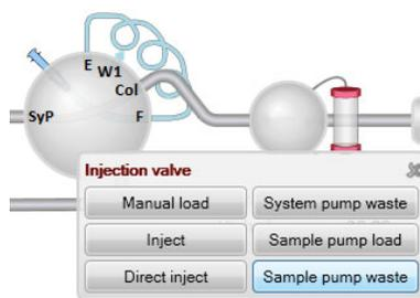
**Result:** The injection valve switches to waste position. This is necessary to achieve a low back pressure during the purge procedure.
