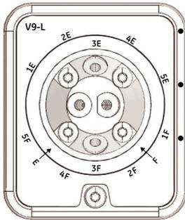
Ports located on the valve head rim are indicated outside the black ring (e.g., 1E, 2E, etc.).
