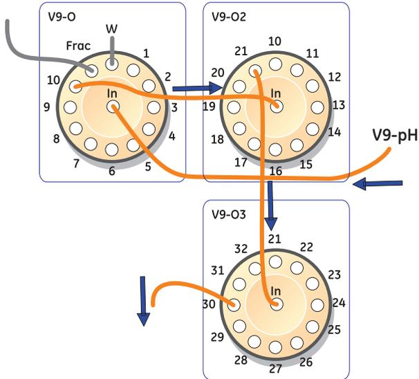
**Note:** The second or third Outlet valve can not be installed together with the second Fraction collector **F9-R**.
