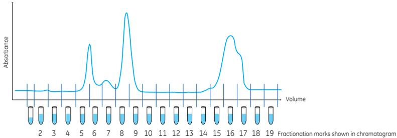
When fixed volume fractionation is used the delay volume is collected at the beginning of fractionation.
