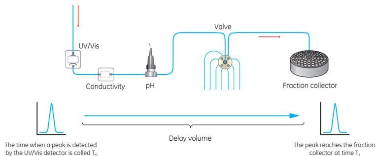
As the delay volume is affected by the length and diameter of the tubing, it should be set according to the tubing and modules used, see [Section 9.12 Delay volumes, on page 500](#).
