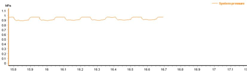
**Incident:** Internal leaking inlet check valve.
