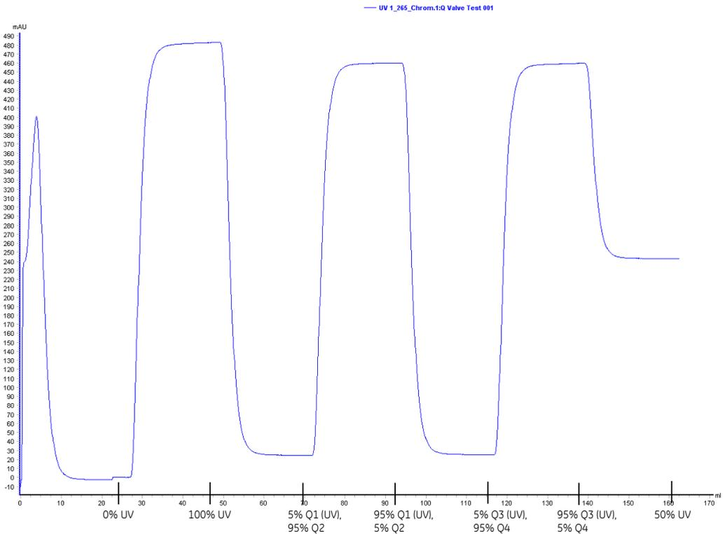
**Note:** The illustration shows a chromatogram from a Q valve test on ÄKTA avant 25. A chromatogram from a Q valve test on ÄKTA avant 150 has a similar appearance, but a different scale on the y-axis.
