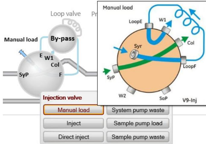
*Result:* The Injection valve switches to **Manual Load** position.
