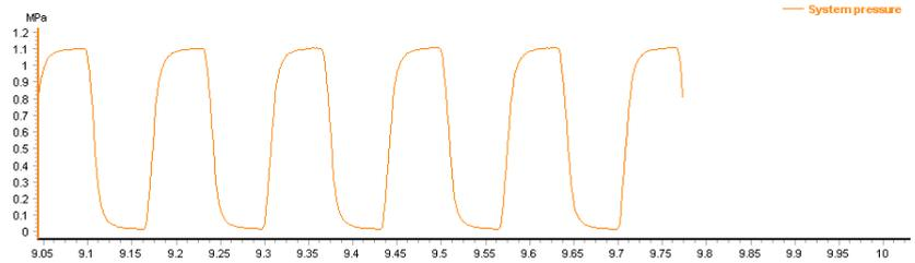
**Incident:** Internal leaking outlet check valve.
