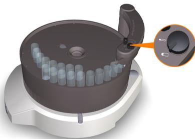
The position for large tubes is used for tubes of approximately 18 mm i.d. and larger. The position for small tubes is used for tubes smaller than 18 mm i.d. Note that this is a rough approximation. Always check that the eluent tubing is centered above the collection tube.
