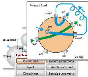
*Result:* Injection valve is set to manual load.
