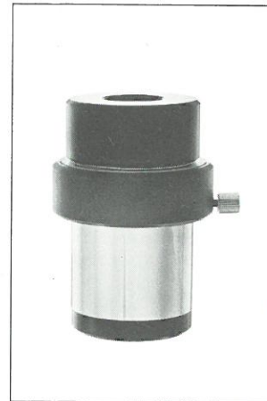
Above: 127 580 Graticule with scale 12 mm : 120
