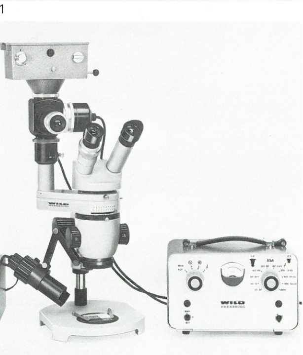
Page 15: M3 Stereomicroscope in trinocular assembly on transmitted-light stand for bright and dark field. Phototube carries attachable camera MKa 1 and 35 mm magazine
