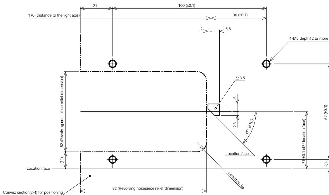
Fix illuminator using four M5 screws and projection for fastening.
