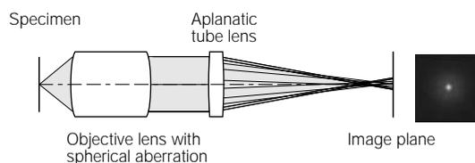
It is said that objective lenses with larger N.A. have better resolution but worsen spherical aberration. Our advanced design and manufacturing techniques have realized good optical performance even with large numerical aperture.
