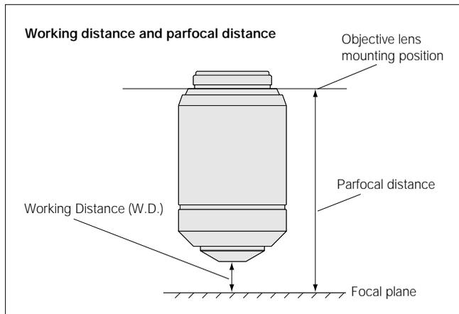
For parfocal distance of the LCPLFLN-LCD series objective lenses, refer to the appropriate objective lens page.
