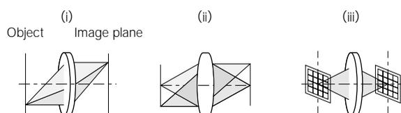
In an actual optical system, however, it is very difficult to strictly meet the requirements for ideal image formation and this causes "aberrations" that interfere with image forming performance.
