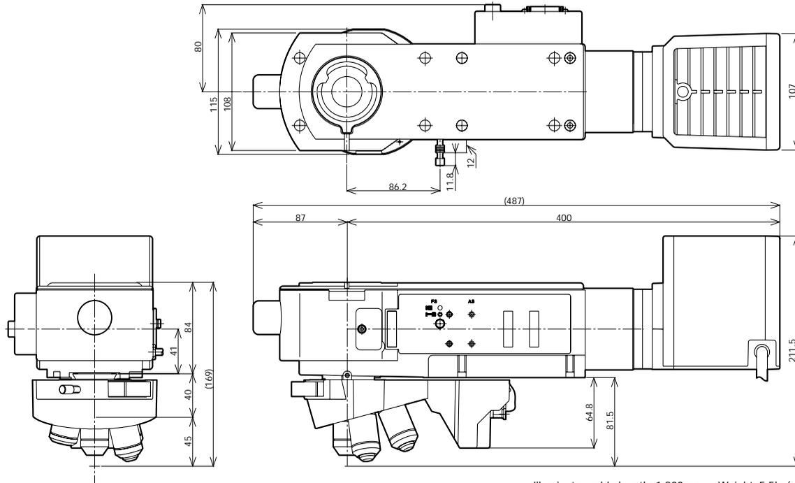
Illuminator cable length: 1.800mm Weight: 5.5kg(exclude objective lens)
