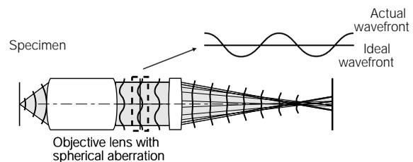
A difference (a degree of disagreement) between the ideal wavefront and the actual wavefront shown above is called "wavefront aberration."
