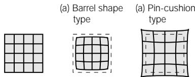
The microscope optical system contains some distortion. When distortion is present, it can bring erroneous results of shape measurements. When a microscope is used for precision measurements, pay close attention to this aberration, for example, by providing it with an aberration compensation function.
