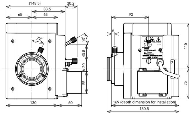
Cable length 2,000mm Accepted lamp: UXL-75XB Weight: 3.1kg
