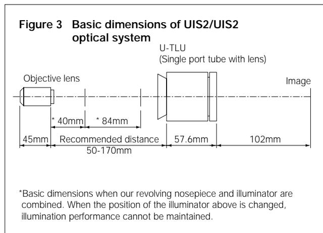
*\*Basic dimensions when our revolving nosepiece and illuminator are combined. When the position of the illuminator above is changed, illumination performance cannot be maintained.*
