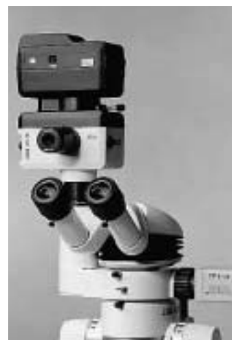
Video/phototube HD, left video/photo objective H, Leica MPS60 camera body. Video objective 0.32× (right) and video module with C-mount
