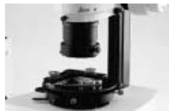
Rotatable polarization stage with sensitive tint-plate, mechanical stage and 360^\circ scale and vernier, analyzer
