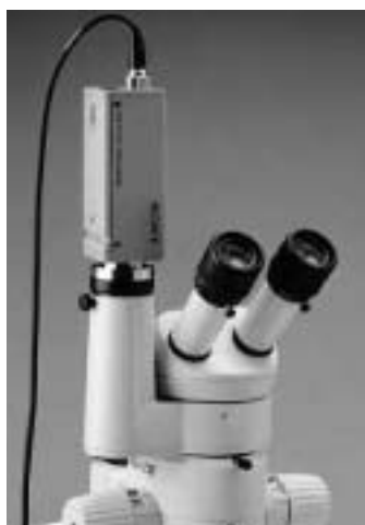
Video/phototube HU with C-mount adapter 0.5× for 1/2" CCD cameras
