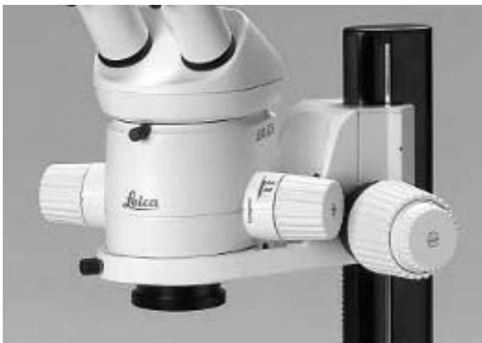
Focusing drive, coarse/fine, for incident-light and transmitted-light stands with side-faced column. Optics carrier in the microscope carrier turned sideways
