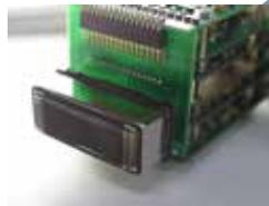
**A microlens array** maximizes photon capture by refocusing light from the prism onto the 32-channel PMT (photomultiplier tube) array.
