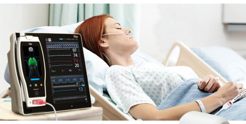
NomoLine infrared sidestream gas analysers provide end-tidal carbon dioxide and multigas measurements (oxygen, nitrous oxide, and anaesthetic gases) in a variety of clinical settings for all patient populations
