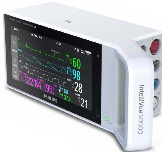
The IntelliVue MX100 monitor provides a comprehensive set of basic physiological measurements, with a color touchscreen display. It can simultaneously monitor ECG (using 3-, 5-, 6- or 10-lead sets, including arrhythmia and ST monitoring), respiration, SpO<sub>2</sub>, NBP, two invasive pressures, temperature, and CO<sub>2</sub>. The multi-touch screen allows easy interaction by swiping and tapping with one or two fingers.
