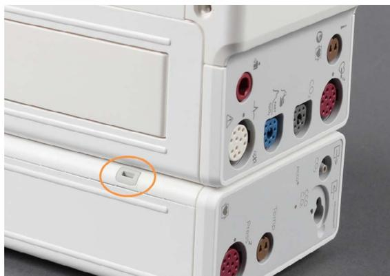
If this is the case, the plugs must be removed with a screwdriver before the measurement extension can be separated from the monitor.
