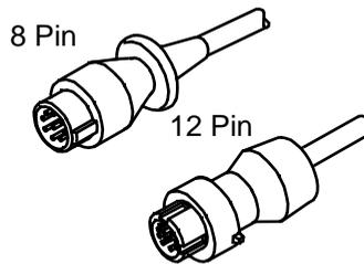
There are four different analog output bedside monitor cables. The cable you use depends upon whether the input connector on your bedside monitor is 8-pin or 12-pin and whether your transmitter lead set is 3- or 5-wire.
