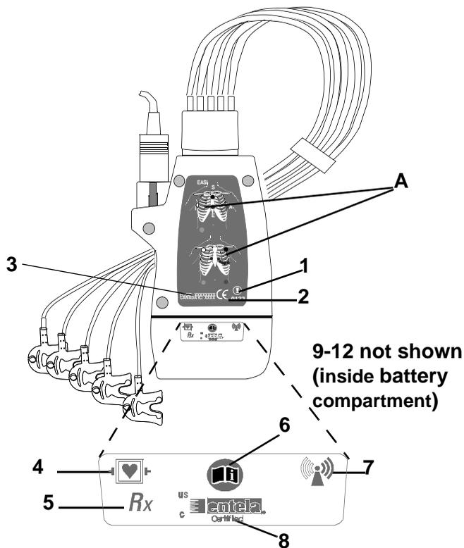
**ECG/SpO<sub>2</sub> Transmitter - Back View**
