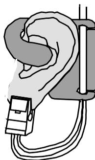
The clip sensor can be used as an alternative if the adult finger sensor does not provide satisfactory results. The preferred application site is the ear lobe, although other application sites with higher perfusion (such as the nostril) can be used. Due to the physiologically lower perfusion in the ear lobe, you should be aware of the reduced accuracy of the measurement and more frequent technical alarms.
