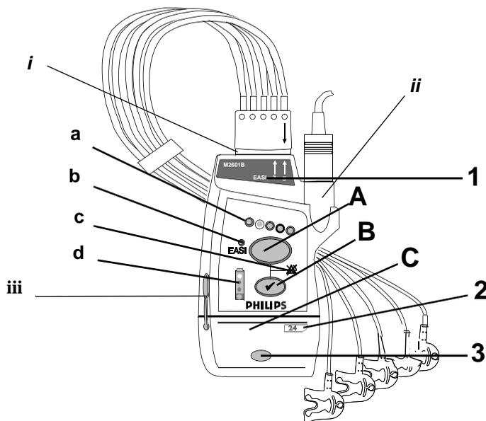
**ECG/SpO<sub>2</sub> Transmitter - Front View**
