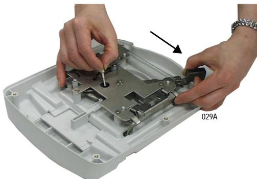
1. Insert the locking lever spring into the spring opening.
