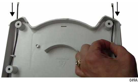
17. If the light pipes are to be replaced, route the light pipes through the bottom housing's LED opening.
