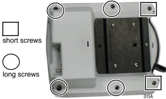
1. Loosen the six screws from the bottom housing.
