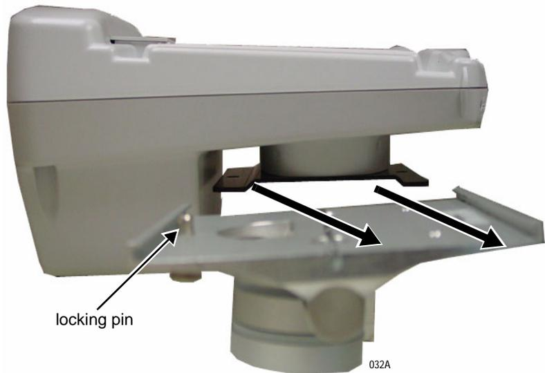
2. Pull down and hold onto the locking pin and continue to slide the docking station onto the GCX mount. Then let go of the locking pin.
