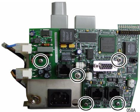
10. Remove the five PCB screws.
