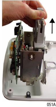
8. Lift out the connector assembly.
