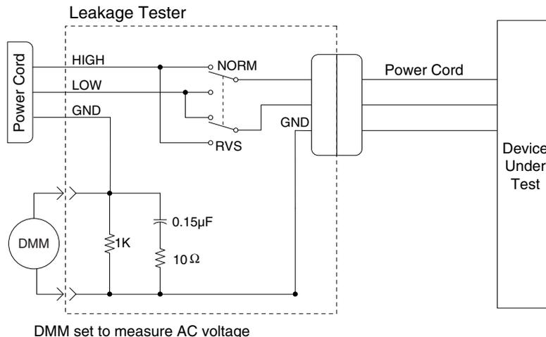
2. Connect the power cord of the device under test to the power receptacle on the leakage tester.
