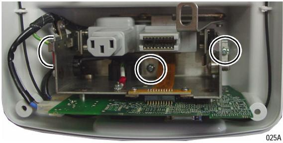
7. Remove the three connector assembly bracket screws from the bottom housing.
