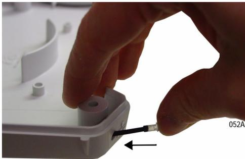
19. Gently push the light pipe lens into the lens opening until it is seated.
