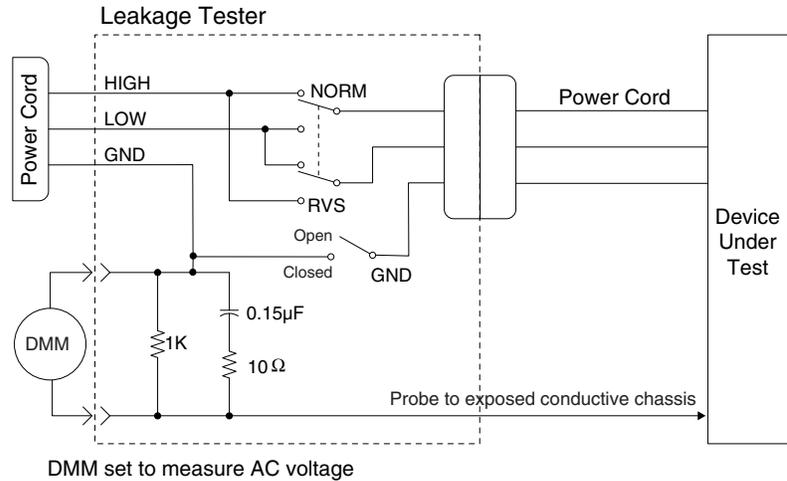
2. Connect probe to an unpainted, non-anodized chassis ground on the unit under test (Equipotential lug).
