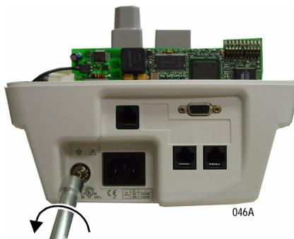
6. Use a 10 mm wrench or nut driver to remove the equipotential lug.
