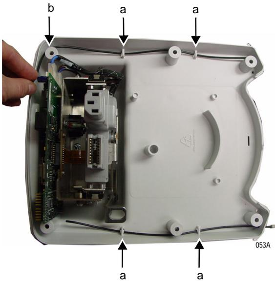
18. Route the light pipes to the PCB light pipe connectors.
