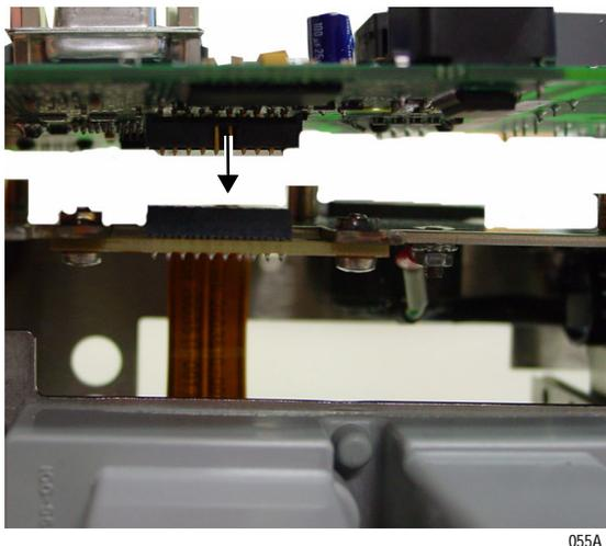
24. Insert the PCB ribbon cable friction connector.
