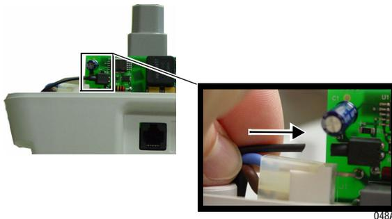
20. Stabilize the PCB LED connector and gently insert the AC power indicator light pipe.
