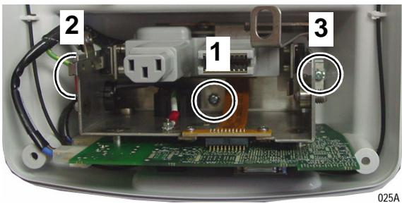
16. Start with the center screw and install the three connector assembly bracket screws.
