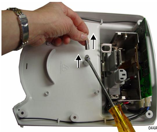
5. Remove the locking lever spring and pin.
