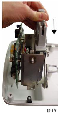
15. Position the replacement Connector Assembly FRU into the bottom housing.
