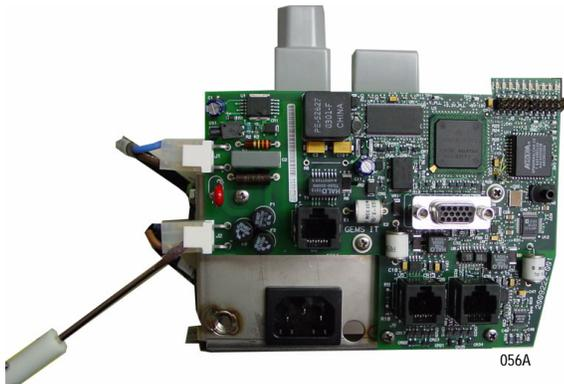
9. Unclip the two power connectors from the PCB.
