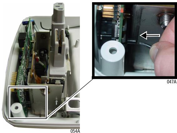
21. Gently insert the communication indicator light pipe into the PCB connector.
