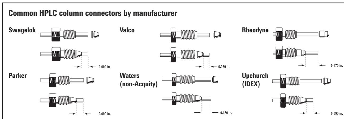
Ideally, you should use the fittings recommended by your column manufacturer. Most analytical reversed-phase columns are compatible with Swagelok or Parker-type fittings when correctly seated in the column.
