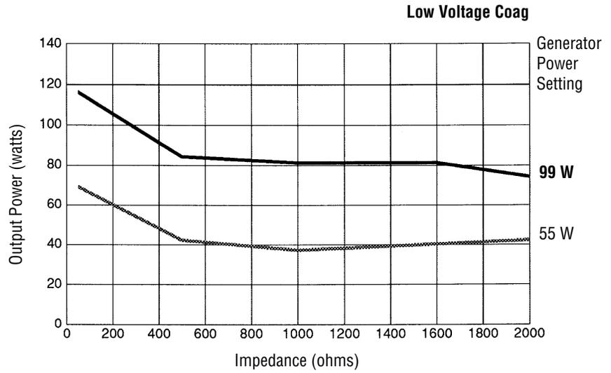
Bipolar measurements are made using bipolar forceps on the insulating surface referred to in IEC 601-2-2, Figure 104.
