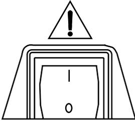
**On/Off Switch** – Press the toggle up to turn power on and down to shut power off.
