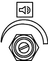
**Audio Volume Control** – When the generator activates, it produces cut, coag, and bipolar mode indicator tones. You adjust the volume of the tones with this control. The volume of the audio alarm is not adjustable.
