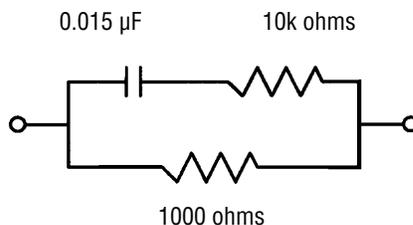
Measure third wire leakage current by opening the green grounding wire at the plug and connecting the 1k ohm resistor from chassis to ground. The maximum voltage across the 1k ohm resistor for 350  $\mu$ A leakage would be 350mV. You may use commercially available leakage testers for this test.
