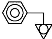
**Equipotential Lug** – You can connect this lug to earth ground with an equipotential grounding cable.
