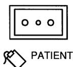
**Patient Return Electrode Receptacle** – This two-pin receptacle accepts the patient return electrode connector you use in monopolar procedures. The receptacle accepts both REM (dual-section) and conventional patient return electrode connectors.
