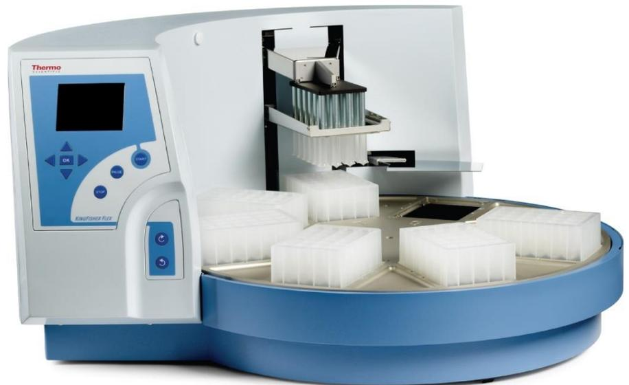
Figure 6. KingFisher Flex magnetic particle processor
