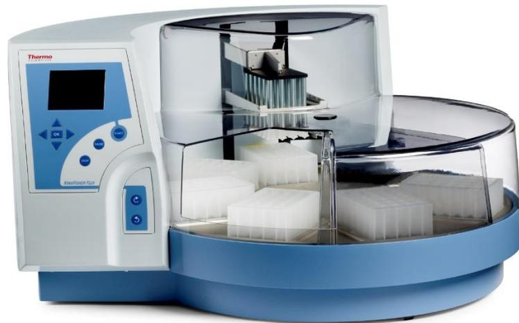
Figure 1. KingFisher Flex magnetic particle processor
