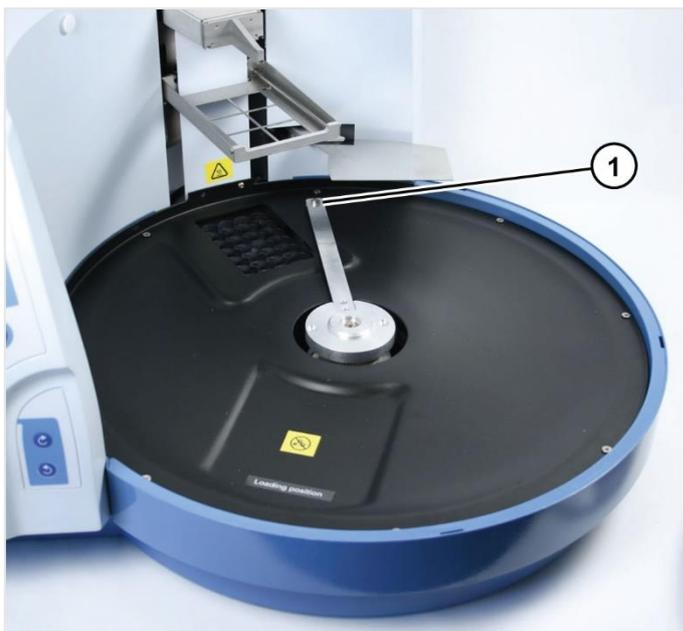
Figure 52. Black spill shield exposed for cleaning
