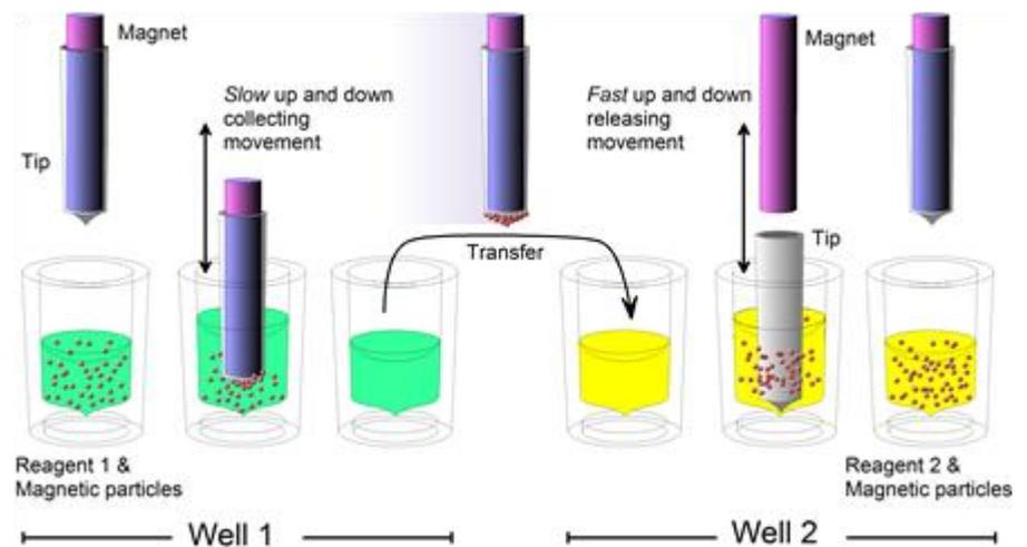
Figure 7. Inverse magnetic particle processing
