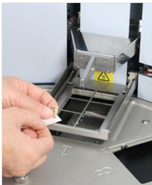
Figure 26. Refit the transport lock of the heating block (A)
