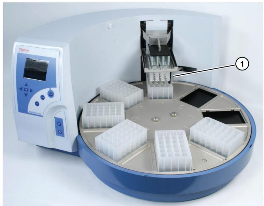
Figure 45. Shield plate in function
