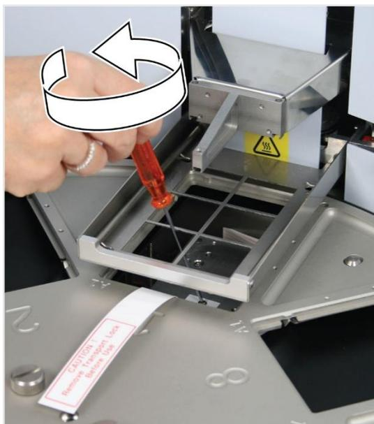
Figure 27. Refit the transport lock of the heating block (B)
