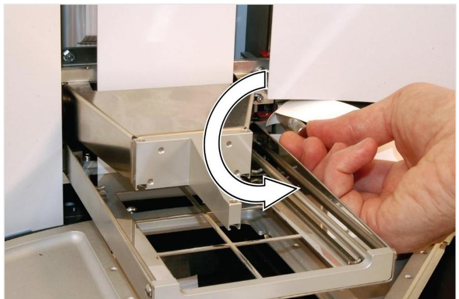
Figure 10. Remove the transport lock of the tip comb holder
