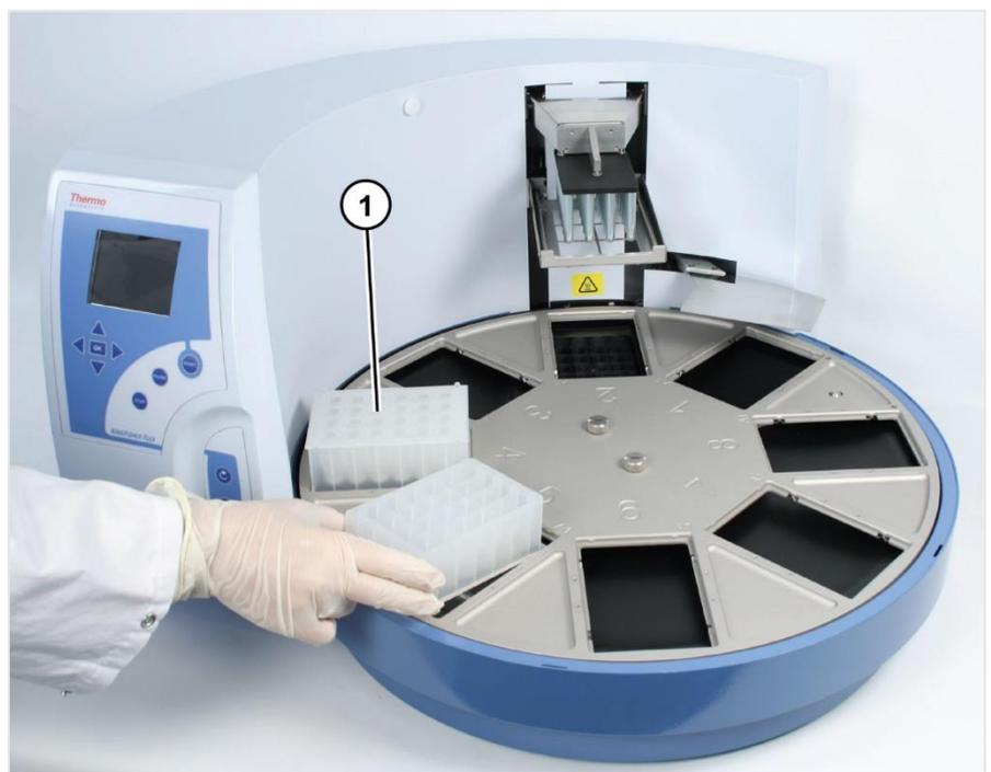
Figure 42. Load the plates
