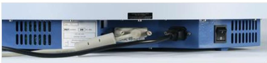
Figure 14. Mains supply cable and serial cable connected
