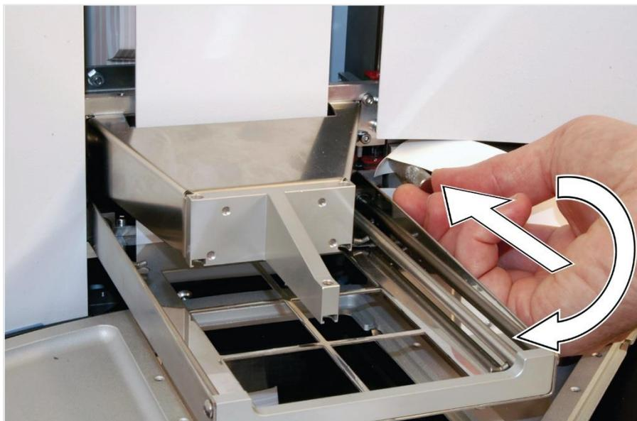
Figure 30. Fit the transport lock of the tip comb holder
