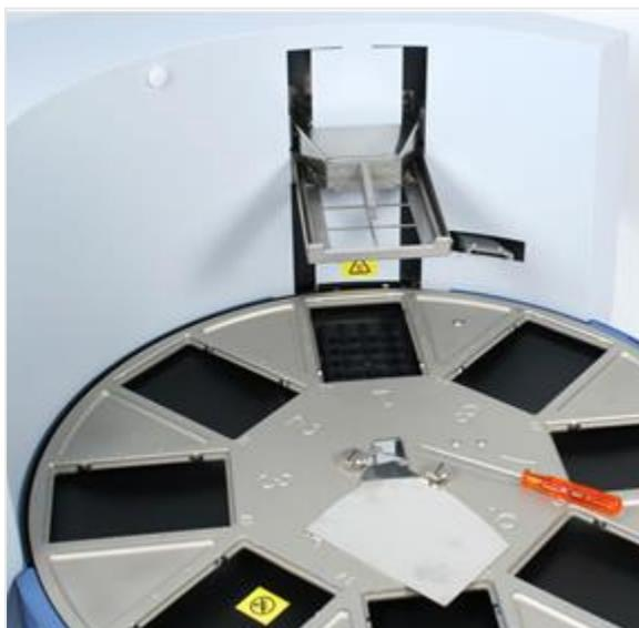
Figure 15. Shield plate prior to fitting
