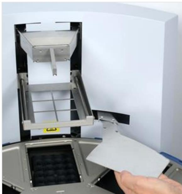
Figure 16. Insert the shield plate
