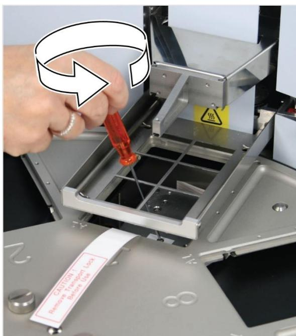
Figure 12. Remove the transport lock of the heating block (A)
