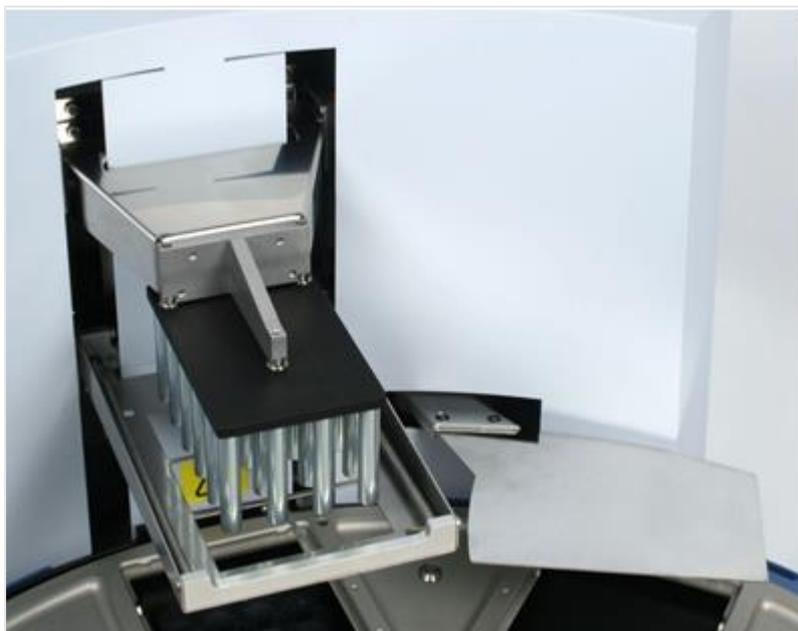
Figure 24. KingFisher Flex head for KingFisher 24 deep well plate fitted
