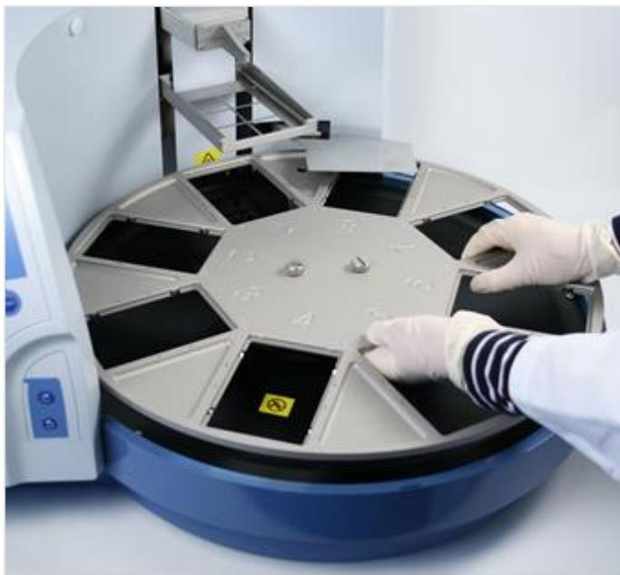
Figure 51. Remove the turntable
