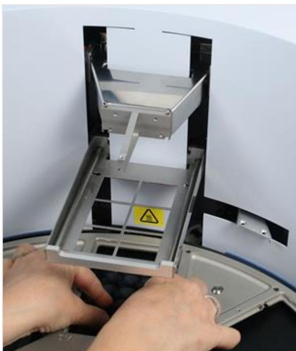
Figure 48. Press the heating block into place
