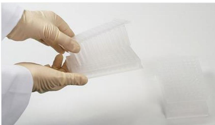
Figure 36. Store the other tip comb on a KingFisher 96 plate for further use
