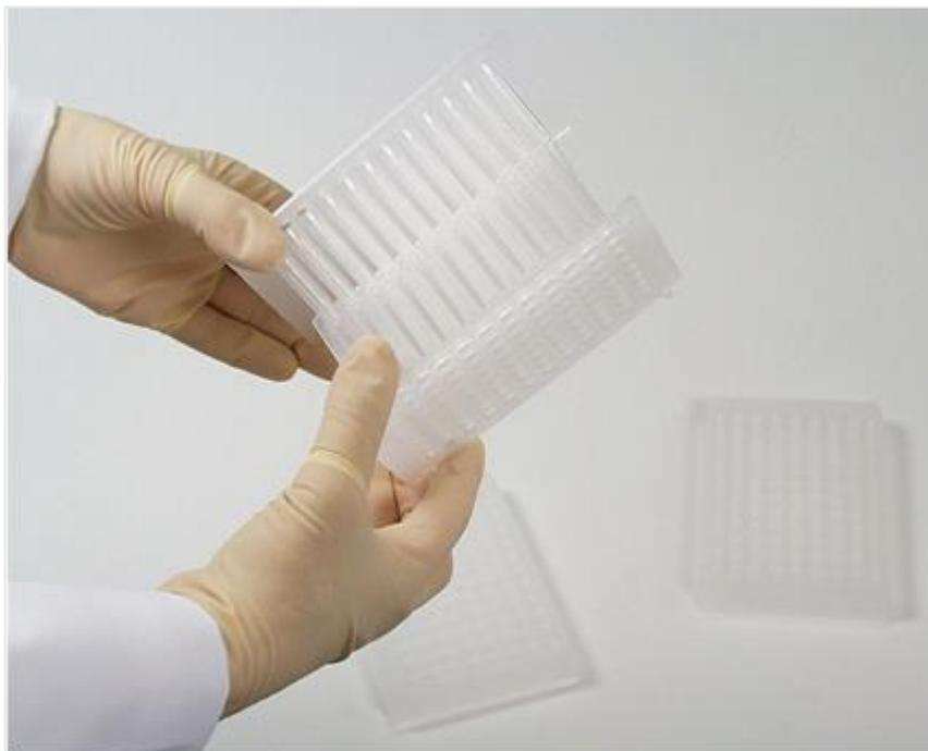
Figure 35. Separate the two tip combs
