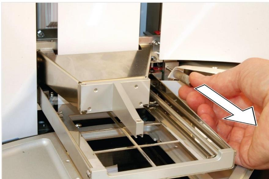
Figure 11. Tip comb holder transport lock removed
