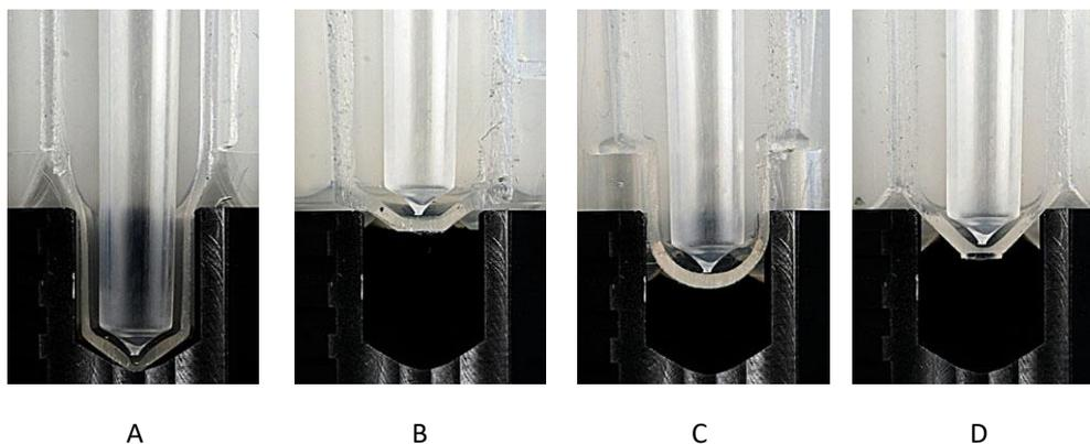
Figure 21. Sectional view of the Microtiter deep well 96 plate (a), deep well 96 plates of other manufacturers (b, c, d) and the KingFisher Flex 96 deep well heating block
