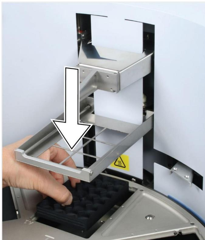
Figure 19. Insert the heating block
