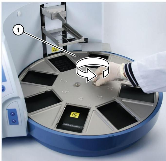
Figure 50. Unfasten the two finger screws
