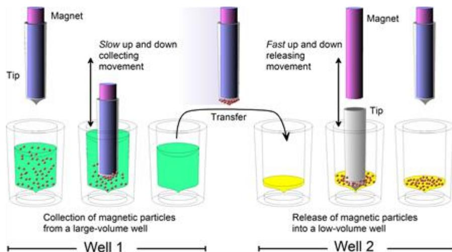
Figure 8. A concentration step during magnetic particle processing
