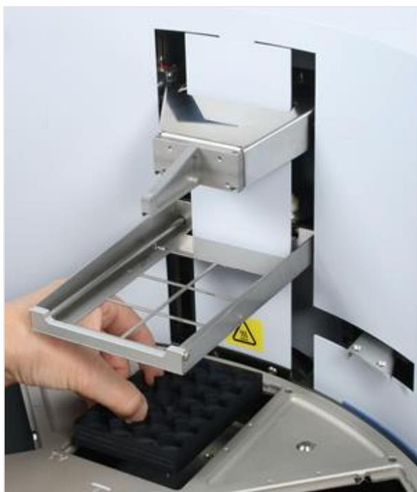
Figure 47. Insert the heating block
