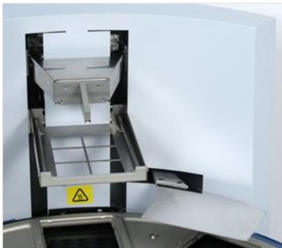
Figure 18. Shield plate fitted
