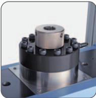
For the range of 1/500 to 1/1 of the load cell rating, a single load cell that guarantees test force accuracy to  $\pm 0.5\%$  of the indicated value (for high-precision type) covers an extensive testing range. The load cell rated value is stored in the calibration cable and automatically recognized when the cable is connected.
