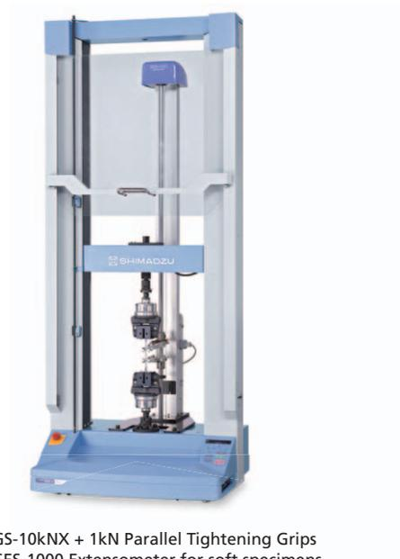
AGS-10kNX + 1kN Parallel Tightening Grips + SES-1000 Extensometer for soft specimens
