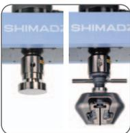
Adopts a single joint for both tension and compression tests. This makes it easier to exchange jigs. In addition, the joint is set with a nut placed in the upper part of the loading cell, which allows for safe detachment of the joint on the table.
