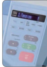
Call up test methods from TRAPEZIUM LITE X to conduct testing. Naturally, AGS-X can be used as a standalone tester to test specimens using methods created with the tester itself.
