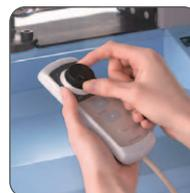
Allows hand-held control of the crosshead position. The jog dial makes fine positioning a breeze, particularly when setting the start position for bending and compression tests.
