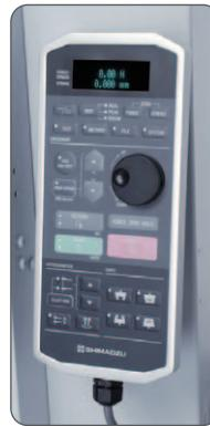
The main operation panel enables the development and storing of test conditions, allowing testing without having to connect to a PC. Perform various operations with the jog wheel, such as opening and shutting the button for automatic grips or the automatic extensometer. The main operational panel is movable, allowing convenient adjustment of the angle.
