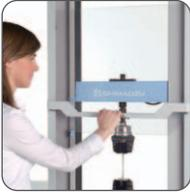
A vertically sliding safety guard is available. Opens easily with one hand. When the safety guard is open, an interlock function disables testing and return movement.
