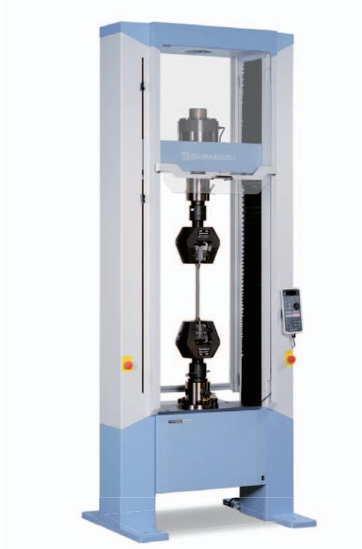
AGS-300kNX + 300kN Non-Shift Wedge Type Grips
