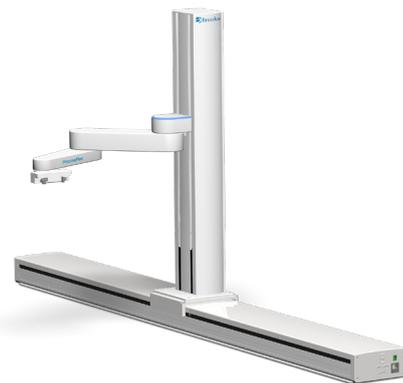
With the vertical column work envelope and embedded controls, PreciseFlex sample handlers offer the highest workspace density, saving valuable floorspace.
