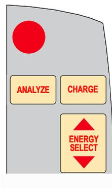
**Note:** If the defibrillator is not discharged within 60 or 120 seconds (user configurable) after reaching the selected energy level, the unit automatically disarms itself.
