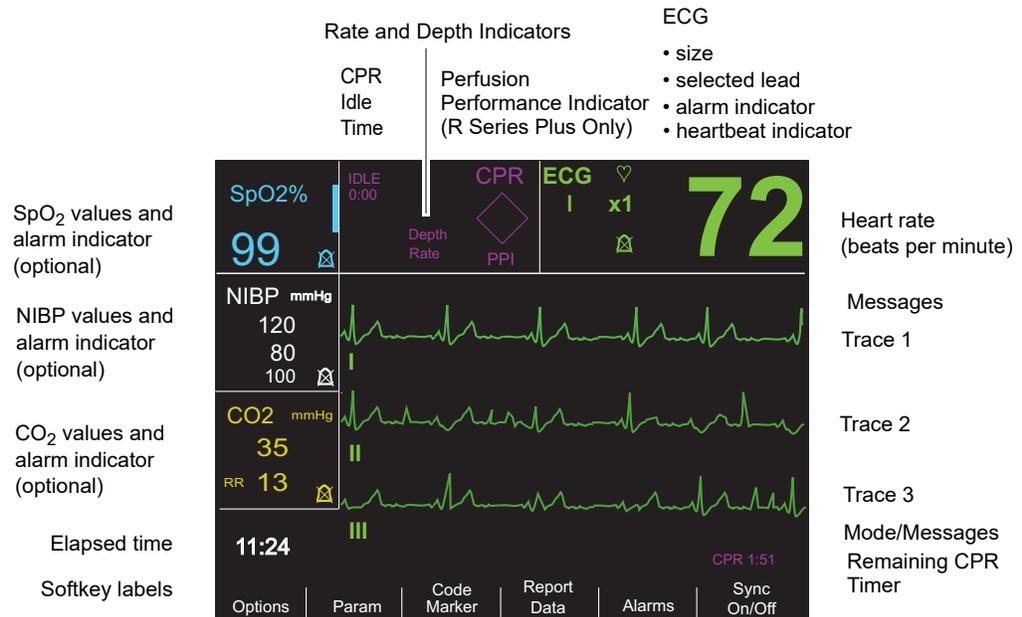
**Figure 2-3. R Series Display Screen (shown in manual mode with optional SpO<sub>2</sub>, NIBP and CO<sub>2</sub> monitoring)**
