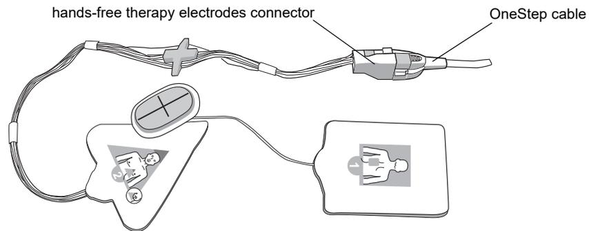
The message *ATTACH PADS* or *CHECK PADS* will be displayed and energy will not be delivered if the therapy electrodes are not making good contact with the patient or if a short circuit exists between the therapy electrodes.
