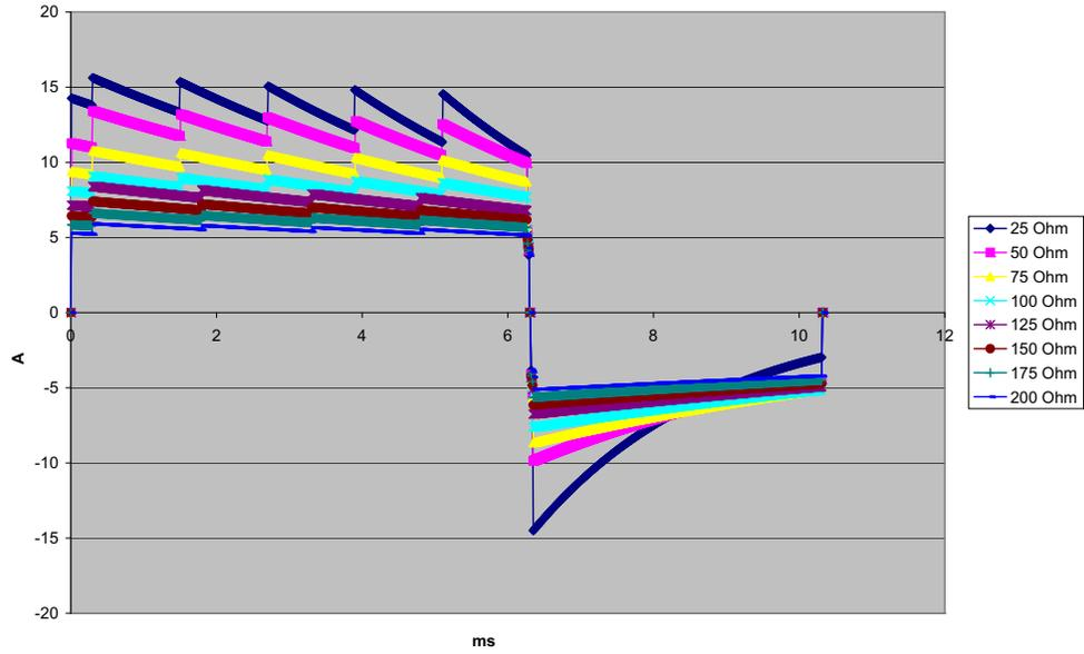
Figure A-8. Rectilinear Biphasic Waveform at 50 Joules
