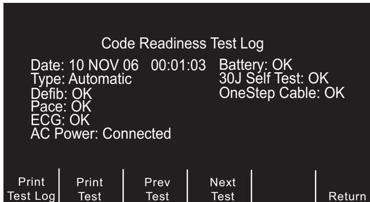
Figure 13-1. Code Readiness Test Log Print Display
