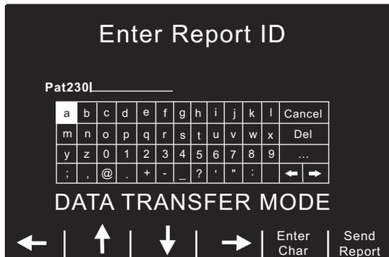
**Note:** Enable Report ID must be enabled in System Configuration mode for the report screen to appear (See the *R Series Configuration Guide*). If Enable Report ID is set to No, then the screen will not be displayed and the report will be sent immediately.
