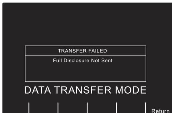
To exit Wi-Fi/DataTransfer Mode, press the **Return** softkey and then the **Exit Transfer** softkey or switch the Mode Selector to **OFF**.
