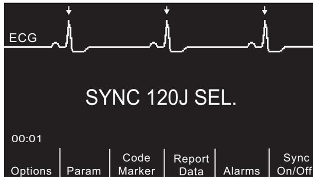
Unless otherwise configured, the unit automatically exits Sync mode after each shock and when the Mode Selector is moved to **PACER** or **OFF**.
