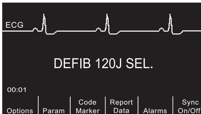
If you have configured Shocks 1, 2, and 3 to escalating energy levels (see the *R Series Configuration Guide* for instructions), the R Series automatically sets the energy to the preconfigured Energy Level: Shock 1, 2, 3 setting at power-up and after each of the first two shocks. The *ENERGY INCREMENTED* message will be displayed after Shocks 1 and 2 are delivered. Manually changing the energy level outside the preprogrammed sequence and delivering a shock disables this function.
