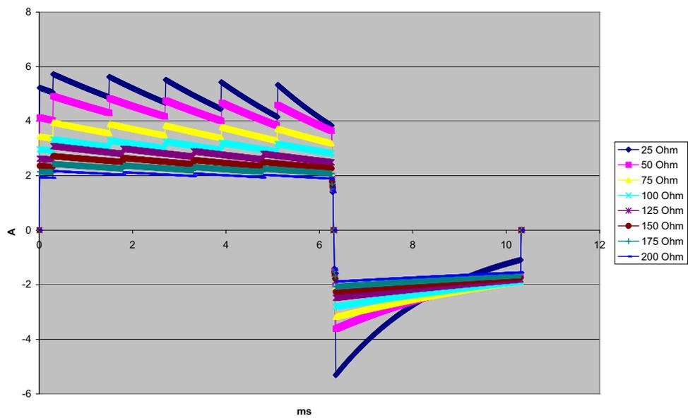
Figure A-15. Rectilinear Biphasic Waveform at 7 Joules
