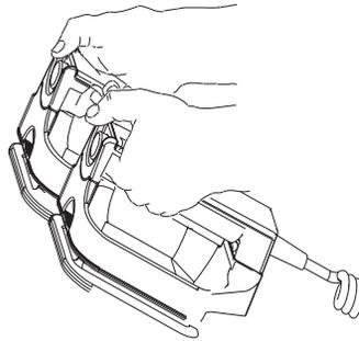
**Caution** Use only thumbs to depress the **SHOCK** buttons. Failure to do so could result in the inadvertent depression of the **ENERGY SELECT** buttons, causing the defibrillator to disarm itself.
