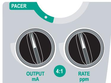
**Note:** When the unit is switched out of PACER mode into Manual mode and then switched back to PACER mode, within 10 minutes the pacer settings remain unchanged.
