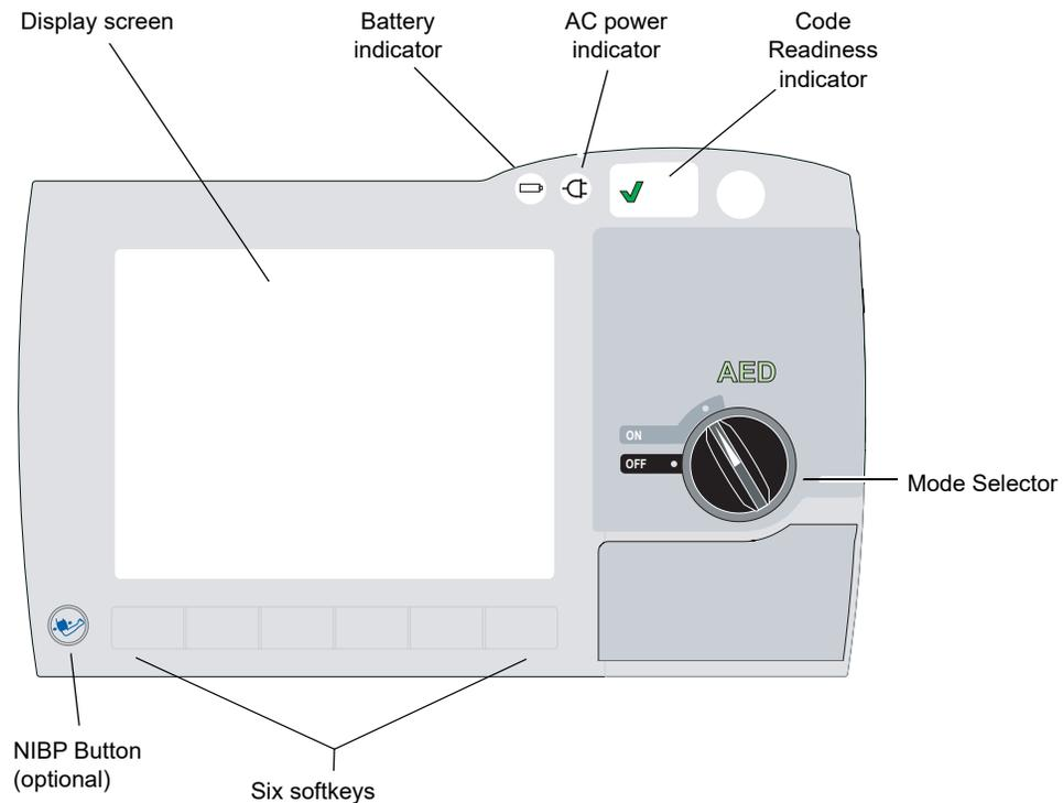
**Figure 2-1. R Series Front Panel (AED Mode)**
