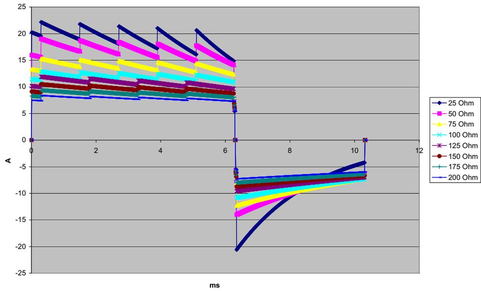
Figure A-4. Rectilinear Biphasic Waveform at 100 Joules
