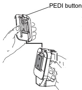
To expose the pediatric plate, press the PEDI button at the top of the paddle, then slide the Adult plate upward. Before replacing the Adult plate, be sure to clean the pediatric plate and surrounding area thoroughly. Slide the Adult plate onto the paddle until it locks into place.
