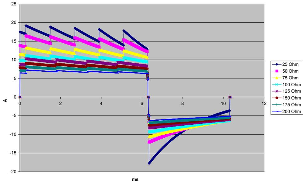
Figure A-6. Rectilinear Biphasic Waveform at 75 Joules
