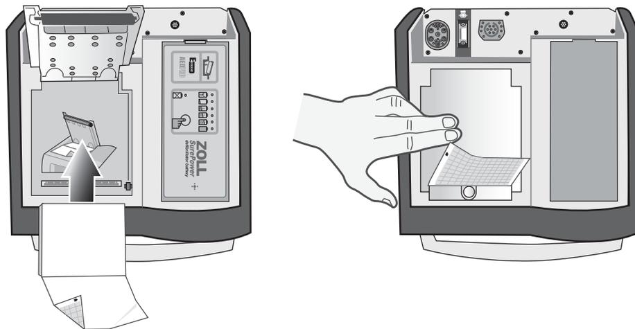
**Figure 13-6. Inserting the Paper and Closing Printer Door**
