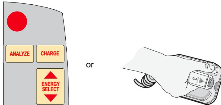
To abort charging and increase or decrease the selected energy after the **CHARGE** button has been pressed, use the **ENERGY SELECT** buttons on either the defibrillator front panel or the sternum paddle. Press the **CHARGE** button again to charge the unit.
