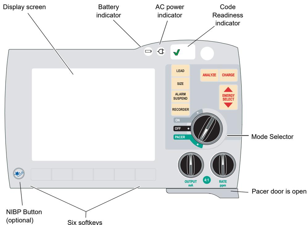
**Figure 2-2. R Series Front Panel (Manual Mode)**
