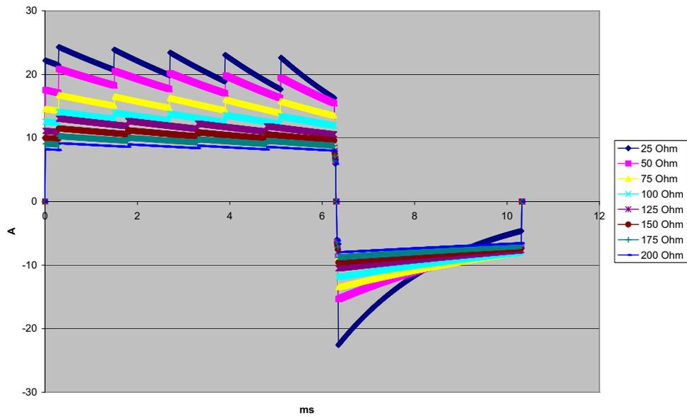
Figure A-3. Rectilinear Biphasic Waveform at 120 Joules
