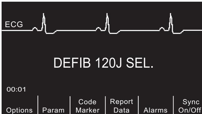
If you have configured SHOCK 1, 2, and 3 to escalating energy levels, and then you manually change the energy level outside preconfigured SHOCK 1, 2, 3 sequence and deliver a shock, it disables the automatic energy escalation. See the Energy Level: Shock 1, 2, 3 section of the *R Series Configuration Guide* for more details.
