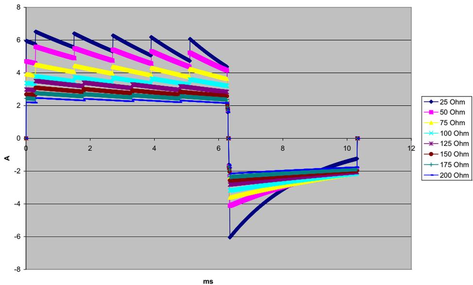
Figure A-13. Rectilinear Biphasic Waveform at 9 Joules
