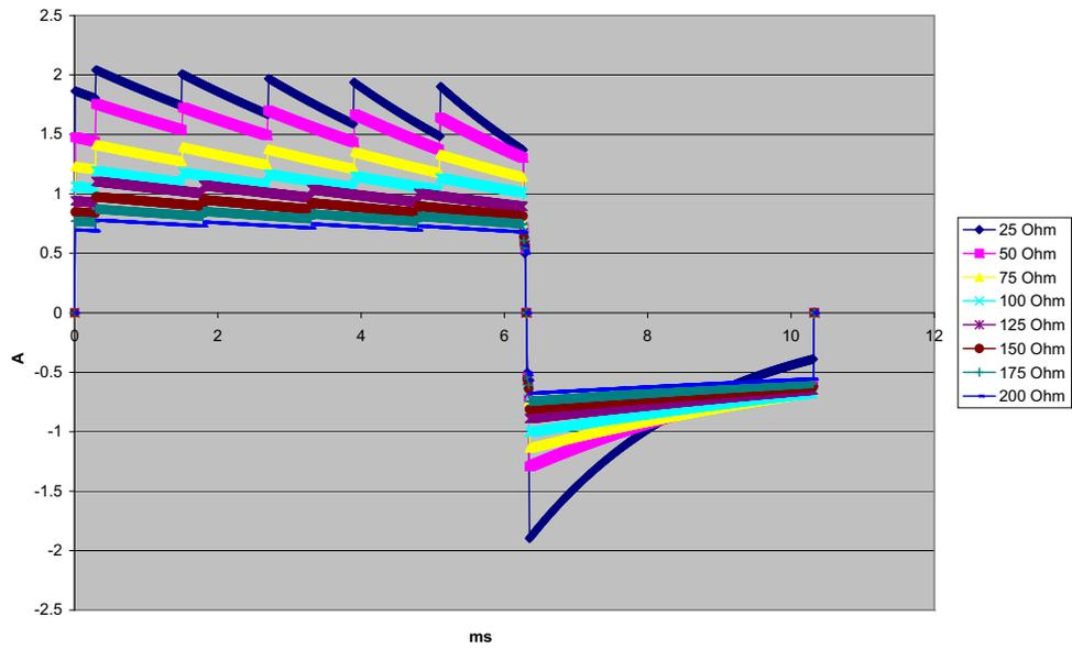
Figure A-21. Rectilinear Biphasic Waveform at 1 Joule
