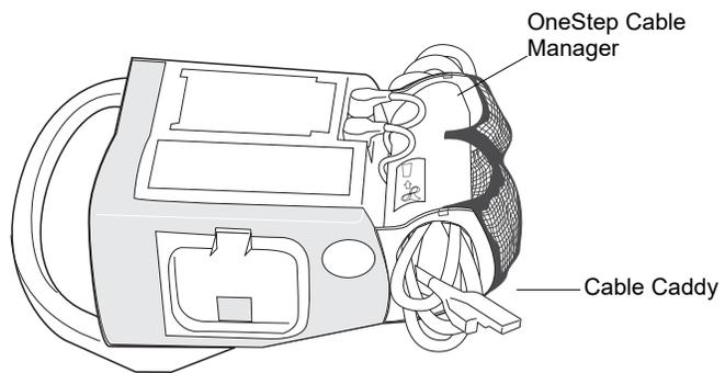
**Figure 2-6. The R Series with the Optional OneStep Cable Manager (Side View)**
