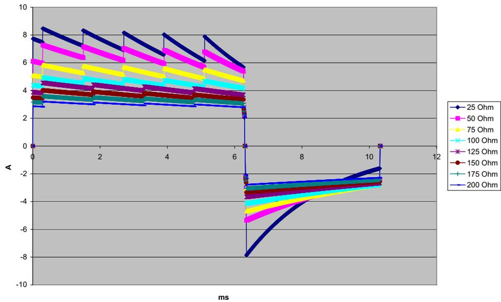
Figure A-11. Rectilinear Biphasic Waveform at 15 Joules
