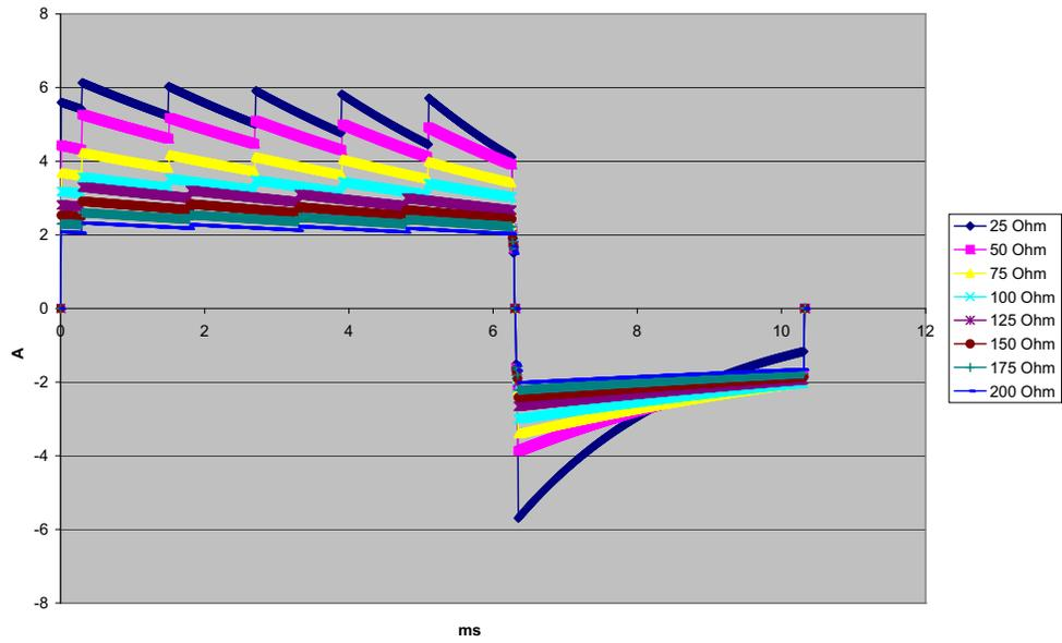
Figure A-14. Rectilinear Biphasic Waveform at 8 Joules
