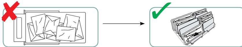
The rack with drying plates will hold 10 autoclave bags. Care must be taken to ensure that the combined weight of the loaded bags does not exceed 1.5 kg (3.3 lbs).
