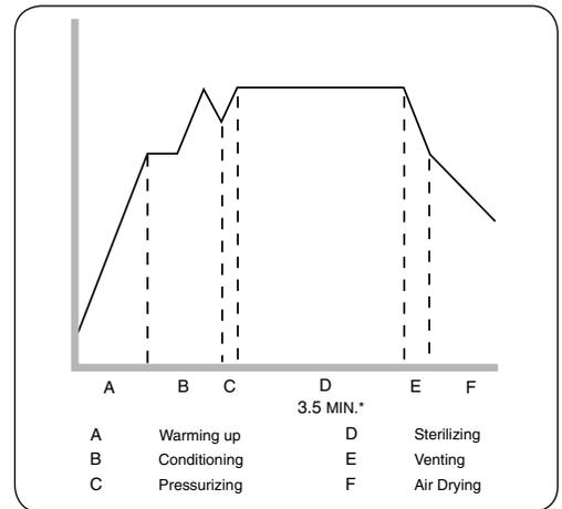
The sterilization temperature in the cassette is 132° C (270° F) and the holding time is 3.5 minutes. See Section STATIM 5000 G4 – Cassette and Section Preparing and Loading Instruments before running this cycle.
