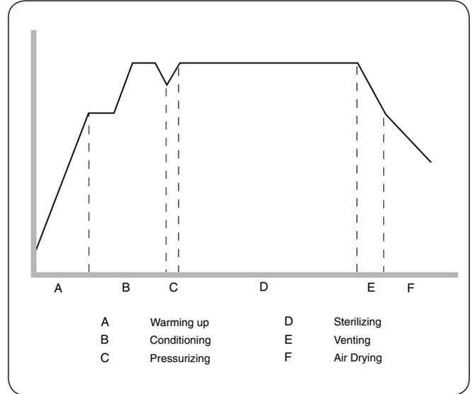
The sterilization temperature in the cassette is 134°C (273°F) and the holding time is 10 minutes. See Section STATIM 2000 G4— Cassette, and Section Preparing and Loading Instruments before running this cycle.
