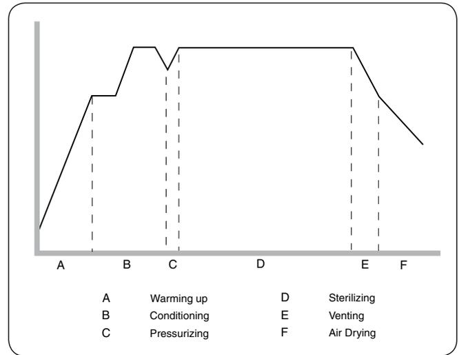
The sterilization temperature in the cassette is 121°C (250°F) and the holding time is 15 minutes.
