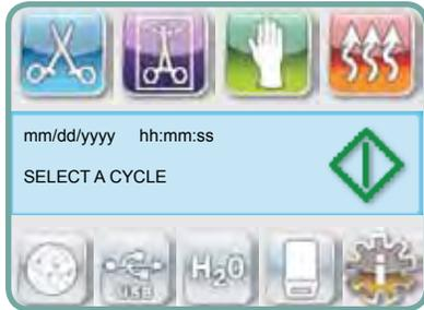
2. Press the appropriate cycle button on the touchscreen. The display will show the cycle name and parameters.
