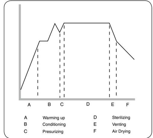
The sterilization temperature in the cassette is 132° C (270° F) and the holding time is 6 minutes.
