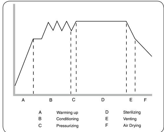
The sterilization temperature in the cassette is 121 °C (250 °C) and for the holding time is 35 minutes.
