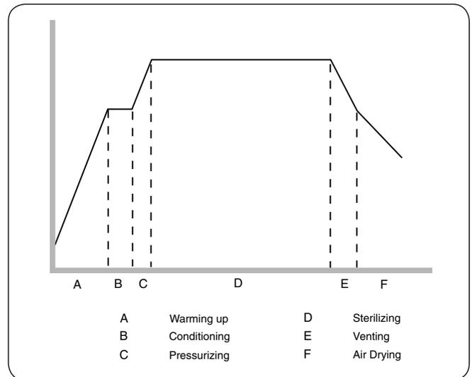
The sterilization temperature in the cassette is 134 °C (273 °F) and the holding time is 3.5 minutes. See Section STATIM 2000 G4 – Cassette, and Section Preparing and Loading Instruments before running this cycle.
