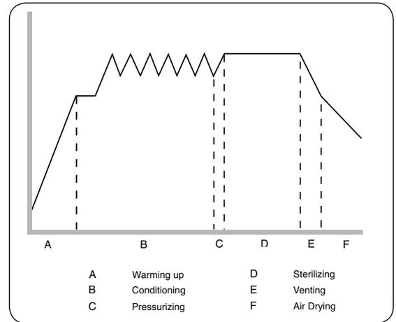
To select the Wrapped Cycle, press the Wrapped Cycle button, then press the START button. The sterilization temperature in the cassette is 132° C (270° F) and the holding time is 6 minutes. See Section STATIM 5000 G4– Cassette and Section Preparing and Loading Instruments before running this cycle.
