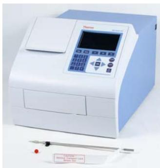
**Figure 3–10.** Transport lock removed
