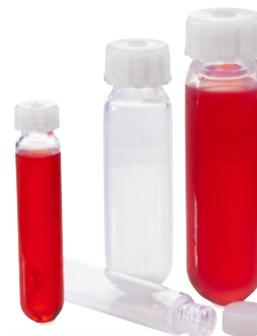
Note: Must be filled to 100% of total capacity for centrifugation.
