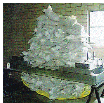
In independent laboratory testing, a BaXstrap was shown to withstand a distributed weight load of greater than 2,500 pounds without permanent structural failure.
