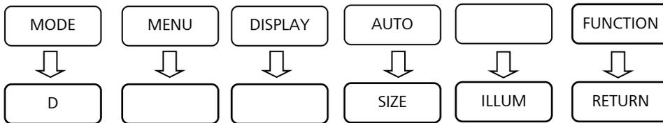
Pressing the **RETURN** key restores the original assignment of function keys.
