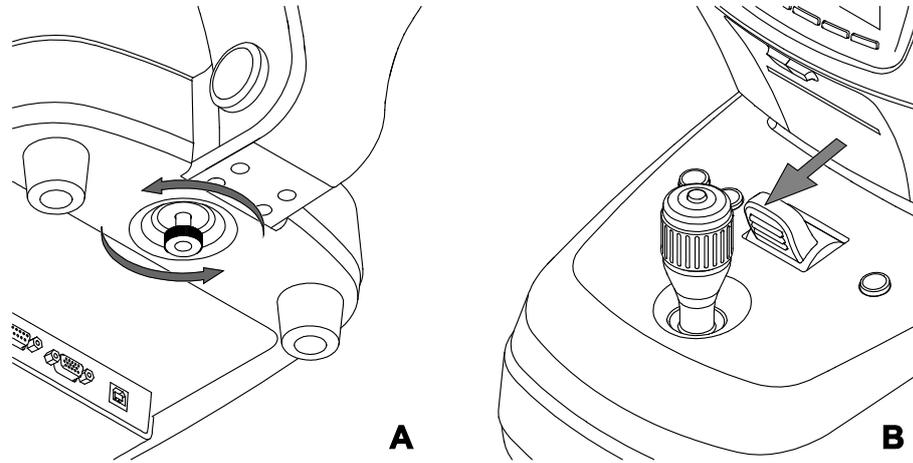
Fig. 7 Releasing the stage locking
