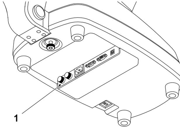
1 Metallic holding plate of plugs (measuring point)
