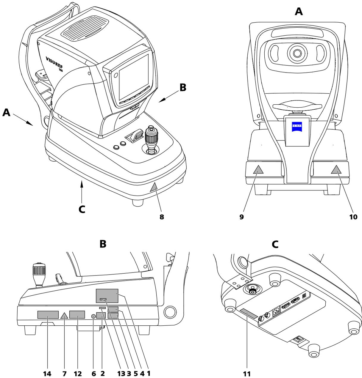
Fig. 2 Labels on the VISUREF 100
