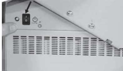
Figure 3: Power Supply Switch Down to Standby
