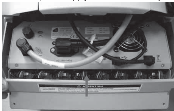
Figure 8: Battery Connector Access Panel - Close
