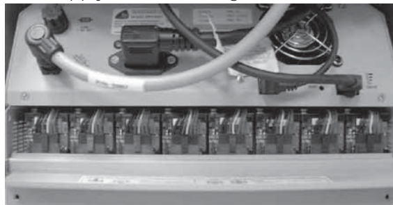
Figure 7: Properly Seated Connections
