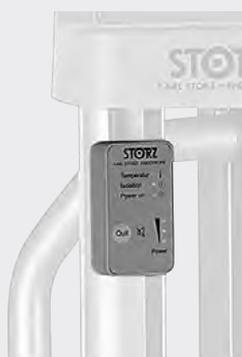
UG 410 **Earth Leakage Monitor**, 200 – 240 V, for mounting to equipment carts, Control panel dimensions: 44 x 80 x 29 mm (w x h x d), for use with Isolation Transformer UG 310
