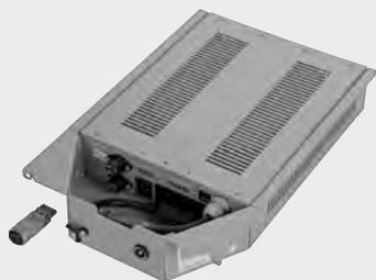
UG 310 **Isolation Transformer**, 200 – 240 V, 2000 VA, with 3 special mains socket, automatic cutout, 3 grounding plugs, Dimensions in mm: 330 x 90 x 495 (w x h x d), for use with Equipment Carts UGxxx
