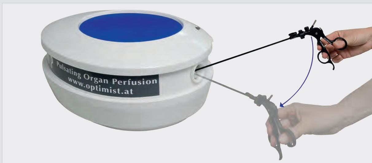
The P.O.P. Trainer DOCK SYSTEM offers the possibility to extend the areas of application for pulsating organ perfusion in the simulation of endoscopic, proctological and endourological OR techniques. The rotating and tilting ball joint enables changing adapters with a diameter of 10 mm to 40 mm.
