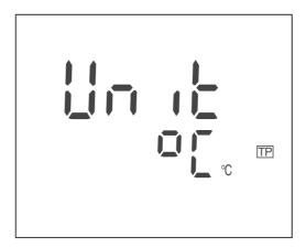
12 Using  $<\Delta><\nabla>$ , toggle between  $^{\circ}C$  and  $^{\circ}F$ .
