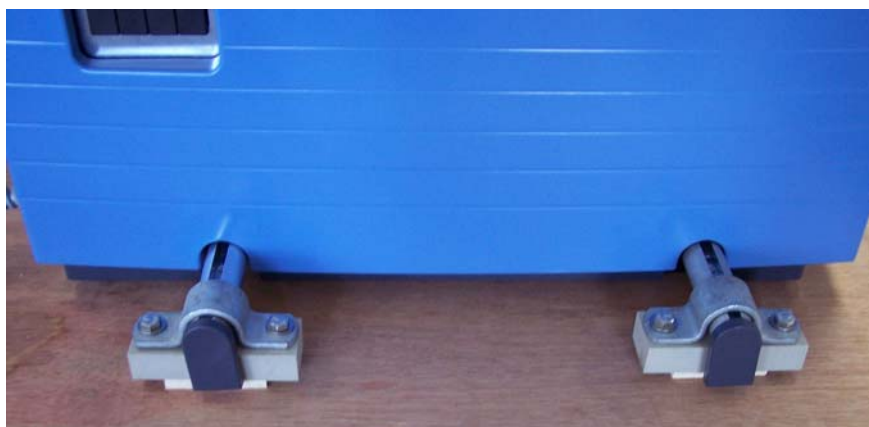
Figure 5-3. Retractable handles for transport, fixed on the transport pallet
