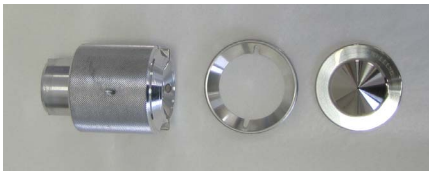
Figure 8-10. Cone tool, sample cone holder and sample cone
