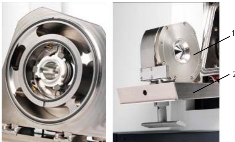
Figure 3-7. Interface with extraction lens and cones
