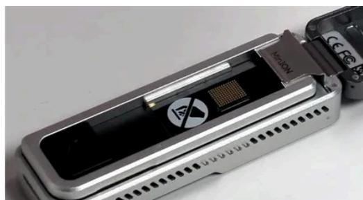
**2 Close the MinION Mk1B lid and connect the MinION Mk1B device to the host computer using the included USB 3.0 cable.**
