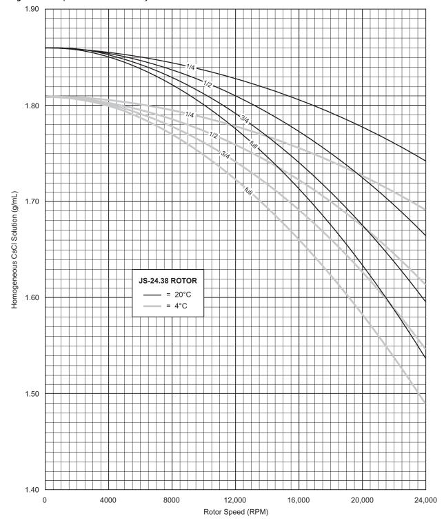
Figure 4 Precipitation Curves for the JS-24.38 Rotor\*
