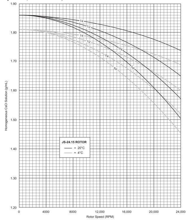
Figure 2 Precipitation Curves for the JS-24.15 Rotor\*
