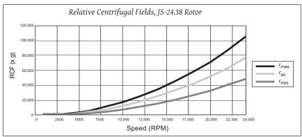
Do not select run speeds in excess of 24,000 RPM in an Avanti JXN-30 or J-30 I; or 10,000 RPM $^*$  in an Avanti JXN-26, J-26S XP series or Avanti J-26 XP series centrifuge. In addition, speeds must be reduced under the following circumstances:
